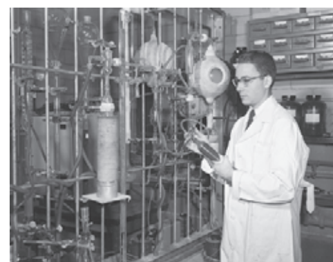
FIGURE 1-34 Abiotic production of biomolecules. (a) Spark-discharge apparatus of the type used by Miller and Urey in experiments demonstrating abiotic formation of organic compounds under primitive atmospheric conditions. After subjection of the gaseous contents of the system to electrical sparks, products were collected by condensation. Biomolecules such as amino acids were among the products. (b) Stanley L. Miller (1930–2007) using his spark-discharge apparatus.
