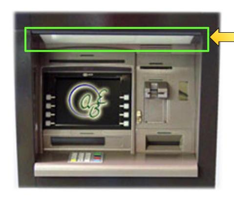
Photo shows a PIN capturing device fitted to the top of the ATM.
