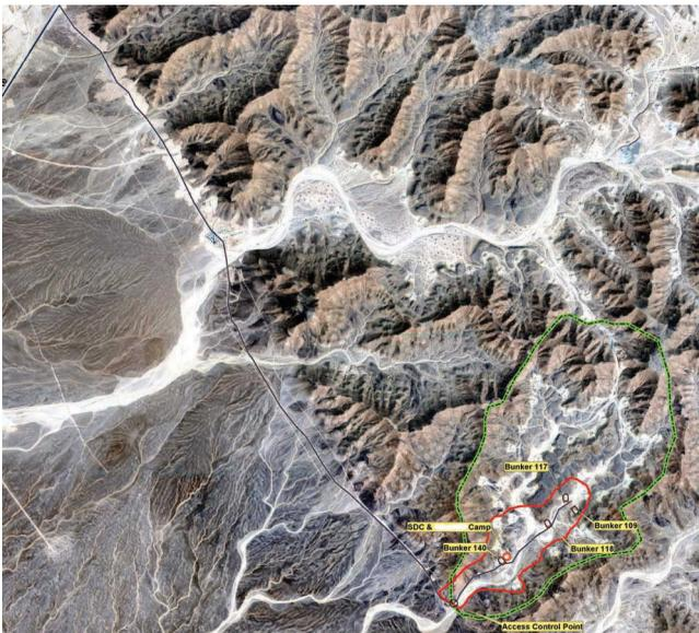
**FIGURE 2.15** Work area and security layout map. The thick green line is the security patrol path. The red line is the work area. The dark purple lines are access roads.
