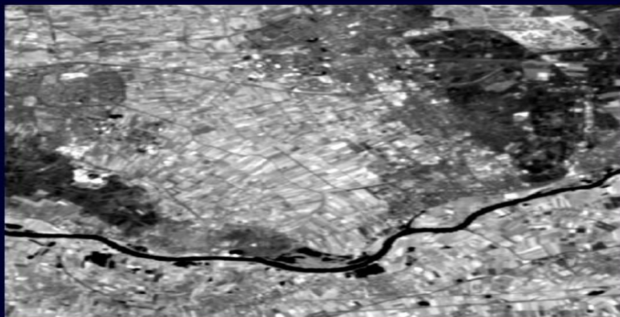
Result low pass filter, 3x3 window
