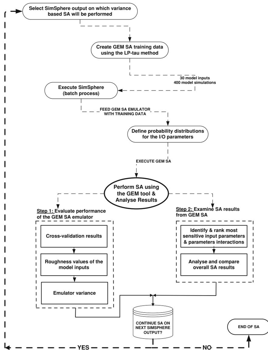
Fig. 2 Flowchart of the overall methodology followed in conducting the GSA on SimSphere using the BACCO method and the GEM SA software platform
