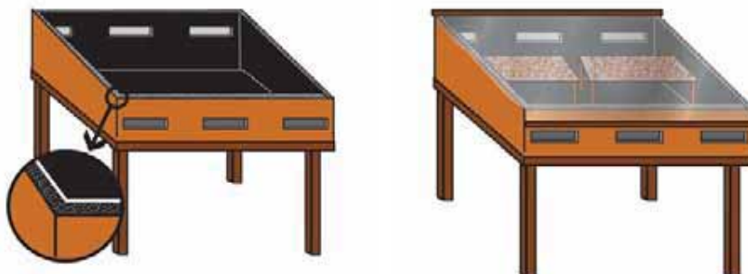
Figure 30: Brace Cabinet Dryer
