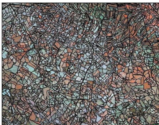
FIGURE 10.4 Segmented image using a scale parameter of 125.
