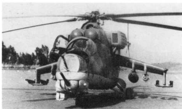
This DRA AF Hind-D was flown to Pakistan by its crew in 1985. The box-like structure above the stub wings is an infra-red suppressor for the engine exhausts, to confuse heat-seeking SAMs. This aircraft carries UV-32 rocket pods and 250kg bombs underwing.
