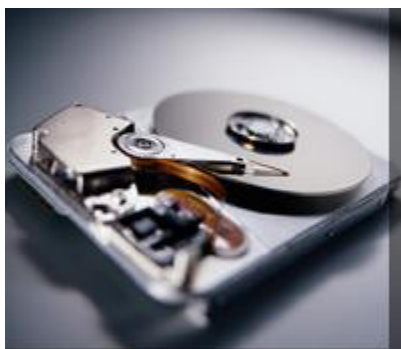
Read/Write Heads and Spindle Motor
