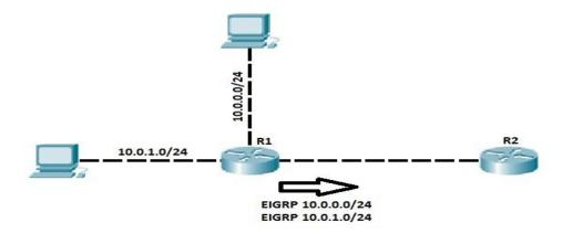
Router R1 and R2 are running EIGRP. Router R1 (on the left) has two directly connected subnets: 10.0.0.0/24 and 10.0.1.0/24. EIGRP advertises these subnets as two separate routes. R2 now has two routes for two subnets, which can be confirmed by using the show ip route command on R2:
