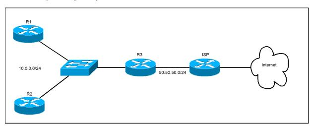
In the network above we have three routers running RIP. Router R3 is connected to the ISP's internet router and and has a static default route that points to it. It is possible to advertise that default route using RIP to other routers in the local network. On R3, we simply need to enter the default-information originate command in the RIP configuration mode.
