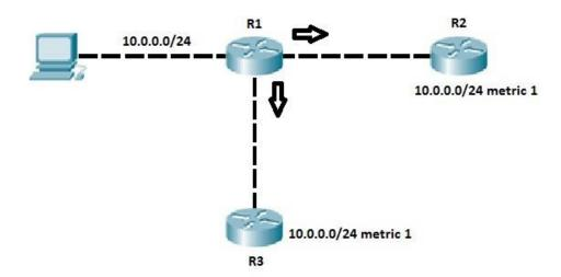
Router R1 directly connects to the subnet 10.0.0.0/24. Network engineer has configured RIP on R1 to advertise the route to this subnet. R1 sends routing updates to R2 and R3. The routing updates list the subnet, subnet mask and metric for this route. Each router, R2 and R3, receives this update and adds the route to their respective routing tables. Both routers list the metric of 1 because the network is only one hop away.
