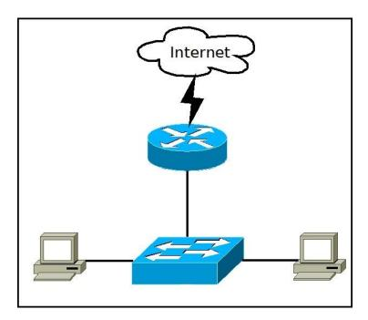
In the picture above we have two computers that are connected to a switch. The switch is then connected to a router that provides the LAN with access to the Internet.
