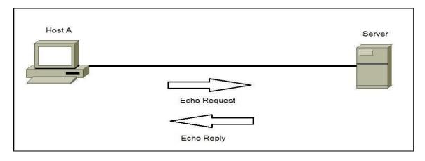
Host A wants to test whether it can reach Server over the network. Host A will start the ping utility that will send ICMP Echo Request packets to Server. If Server is reachable, it will respond with ICMP Echo Reply packets. If Host A receives no response from Server, there might be a problem on the network.
