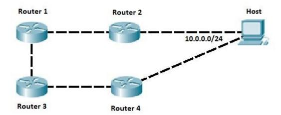
RIP has been configured on all routers. Router 1 has two paths to reach the subnet 10.0.0.0/24. One path is goes through Router 2, while the other path goes through Router 3 and then Router 4. Because RIP uses the hop count as its metric, the path through Router 1 will be used to reach the 10.0.0/24 subnet. This is because that subnet is only one router away on the path. The other path will have a higher metric of 2, because the subnet is two routers away.
