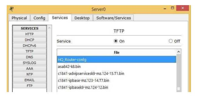
To backup the startup configuration to a TFTP server, you can use the copy startup-config tftp: command:
