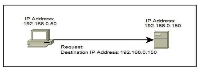
In the picture above you can see that the host wants to communicate with the server. It uses the (unicast) IP address of the server (192.168.0.150) to do so.
