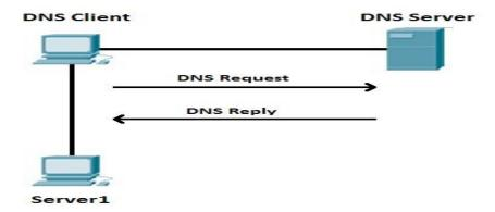
Suppose that the DNS Client wants to communicate with the server named Server1. Since the DNS Client doesn't know the IP address of Server1, it sends a DNS Request to the DNS Server, asking for Server1's IP address. The DNS Server replies with the IP address of Server1 (DNS Reply).
