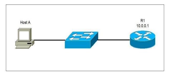
A user wants to transfer files from Host A to the router R1. R1 is a Cisco device and it has a TFTP server installed. The user will start an TFTP client program and initiate the data transfer.
