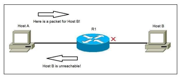
Host A sends a packet to Host B. Because the Host B is down, the router will send an ICMP Destination host unreachable message to Host A, informing it that the destination host is unreachable, e.g.:
