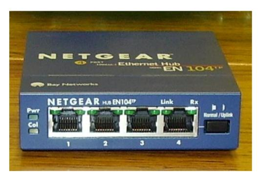
Today, hubs are considered obsolete and switches are commonly used instead. Hubs have numerous disadvantages. They are not aware of the traffic that passes through them. They create only one large collision domain. A hub typically operates in half duplex. There is also a security issue with hubs since the traffic is forwarded to all ports (except the source port), which makes it possible to capture all traffic on a network with a network sniffer!
