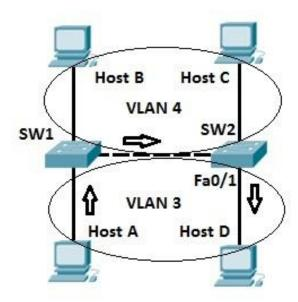
On the segment between two switches, a process called VLAN trunking is used. Let's say that host A sends a broadcast frame. SW1 "tags" the frame by inserting the VLAN ID in the header of the frame before sending the frame to SW2. SW2 receives the frame and knows that the frame belongs to VLAN 3, so it sends the frame only to host D, since that host is in VLAN 3.
