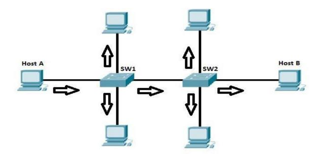
Without VLANs, a broadcast sent from host A would reach all devices on the network. By placing interfaces Fa0/0 and Fa0/1 on both switches into a separate VLAN, a broadcast from host A would reach only host B, since each VLAN is a separate broadcast domain and only host B is inside the same VLAN as
