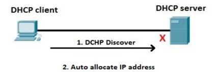
The host on the left is configured as DHCP client. The host boots up and looks for DHCP servers on the network. However, the DHCP server is down and can't respond to the host. After some time (from a couple of seconds to a couple of minutes, depending on the operating system) the client auto-configures itself with an address from the APIPA range (e.g. 169.254.154.22).
