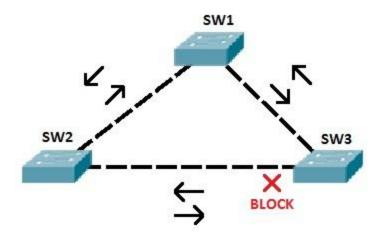
In the topology above, STP has placed one port on SW3 into the blocking state. That way, if SW3 receives a broadcast frame from SW1, it will not forward it out the port connected to SW2.
