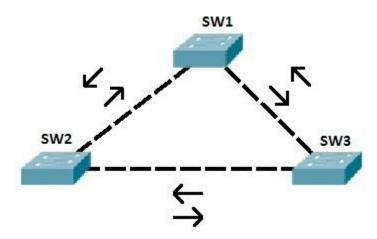
SW2 sends a broadcast frame to SW1 and SW3. Both switches receive the frame and forward the frame out every port, except the port the frame was received on. SW1 sends the frame to SW3. SW3 receives the frame, and sends the frame back to SW2. SW2 then again forwards the frame to SW1! The same thing also happens in the opposite direction. Without STP in place, these frames would loop forever. STP prevents loops by placing one of the switch ports into blocking state.
