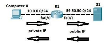
Computer A requests a web resource from S1. Computer A uses its private IP address when sending the request to router R1. Router R1 receives the request, changes the private IP address to the public one and sends the request to S1. S1 responds to R1. R1 receives the response, looks up in its NAT table and changes the destination IP address to the private IP address of Computer A.
