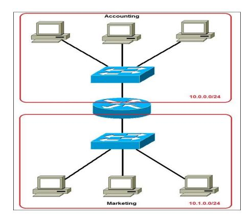
Now, two subnets were created for different departments: 10.0.0.0/24 for Accounting and 10.1.0.0/24 for Marketing. Devices in each subnet are now in a different broadcast domain. This will reduce the amount of traffic flowing on the network and allow us to implement packet filtering on the router.
