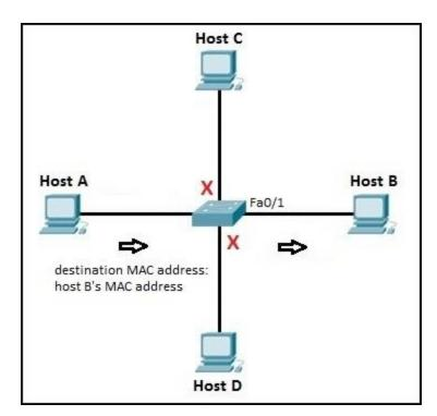
You can display the MAC address table of the switch by using the show mac-address-table command:
