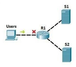
In the example network above, we have used the standard access list to prevent all users to access server S1. But, with that configuration, we have also disable access to S2! To be more specific, we can use extended access lists. Let's say that we need to prevent users from accessing server S1. We could place an extended access list on R1 to prevent users only from accessing S1
