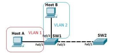
Host A and host B are in different VLANs, VLAN 1 and VLAN 2. These ports need to be configured as access ports and assigned to their respective VLANs by using the following sequence of commands:
