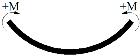
positive moment concave upward
