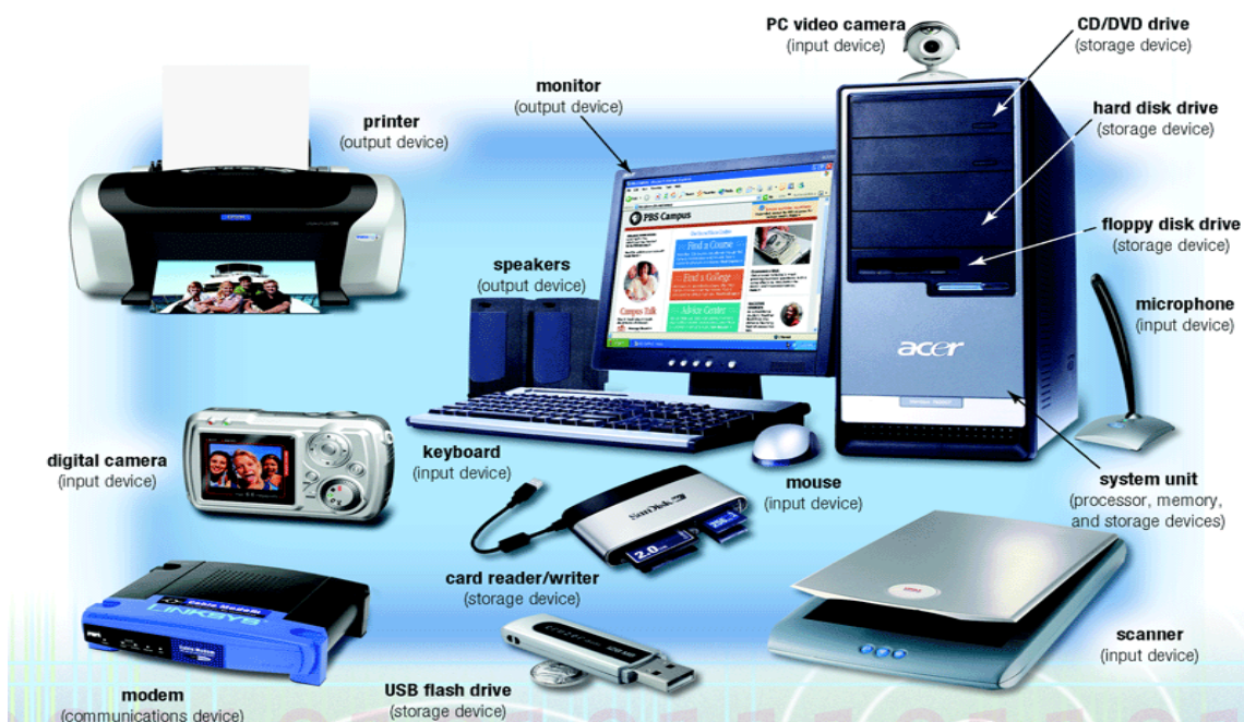
FIGURE 1 Common computer hardware components.
