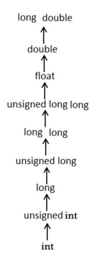
The usual arithmetic conversions are not performed for the assignment operators, nor for the logical operators && and ||. Let us take the following example to understand the concept:
