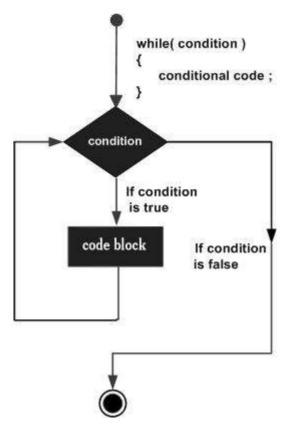
Here, the key point to note is that a while loop might not execute at all. When the condition is tested and the result is false, the loop body will be skipped and the first statement after the while loop will be executed.
