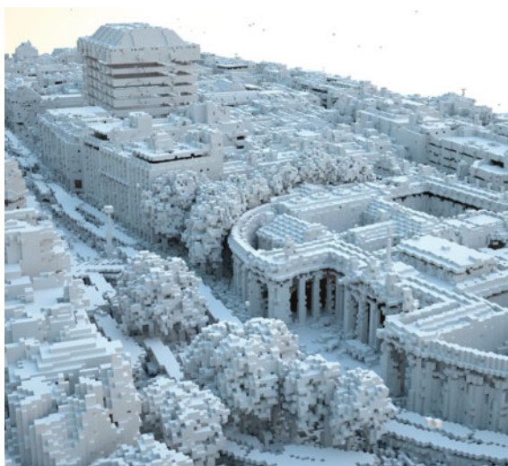
Fig. 11 Voxelization of laser scanning points shows an automated strategy for point conversion into a solid model
