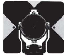
FIGURE 8.6 Typical standard prism and sight
