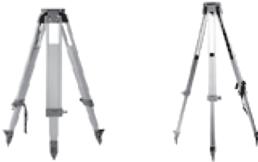
FIGURE 8.5 Wooden and aluminium tripods for total station
