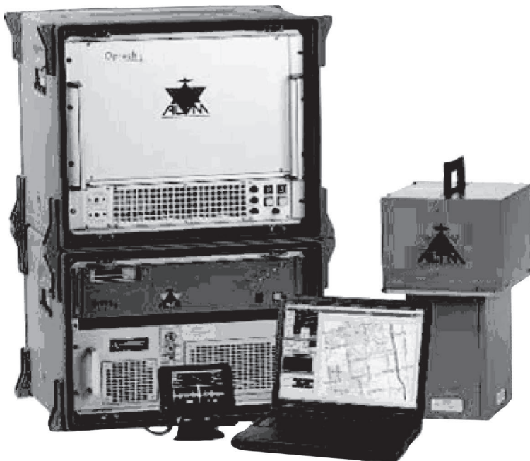
FIGURE 13.22 OPTECH 2050 LIDAR equipment operated by laser map
