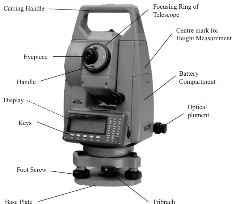
FIGURE 10.4 Parts of a total station
