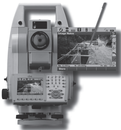
FIGURE 8.13 An imaging total station (courtesy of Leica)
