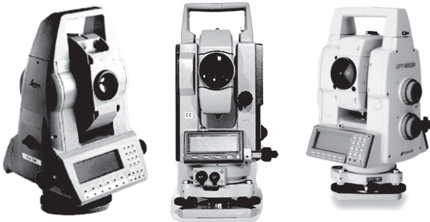
FIGURE 8.4 Different models of total station
