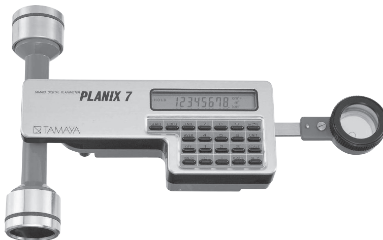
FIGURE 12.9 Digital planimeter (electronic rolling planimeter Courtesy M/S.Sokkia)
