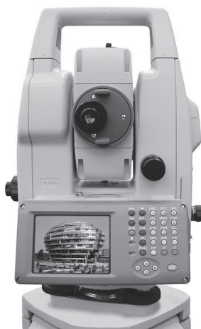
FIGURE 8.12 An imaging total station (courtesy of Sokkia)
