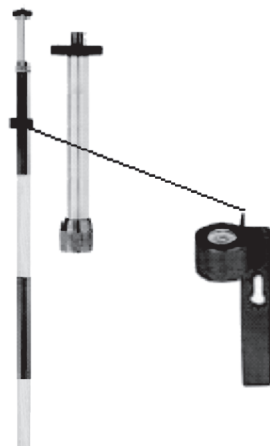
FIGURE 8.7 Typical standard rod (with bubble level)
