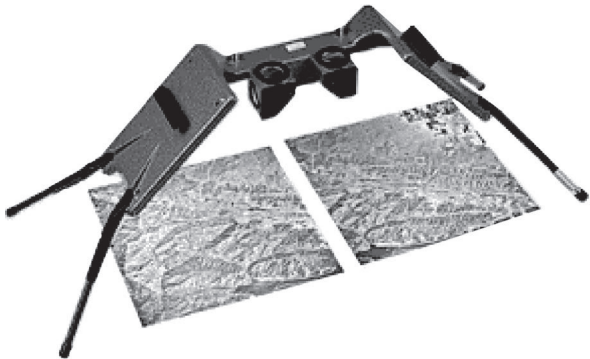
FIGURE 13.15 A mirror stereoscope
