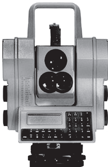
FIGURE 8.3 An old model total station
