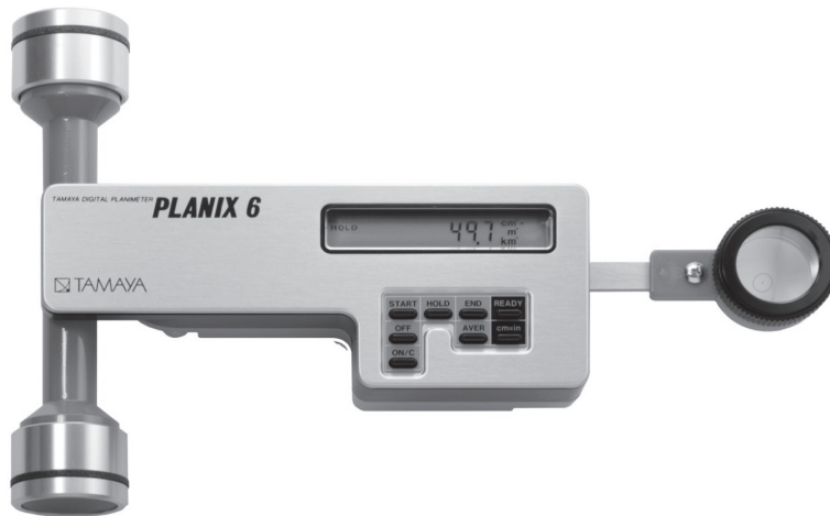
FIGURE 12.10 Digital planimeter (courtesy M/S.Sokkia)
