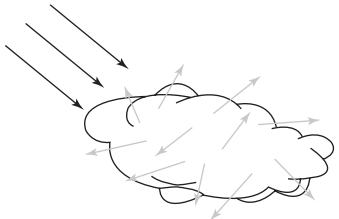
FIGURE 14.7 Scattering of waves
