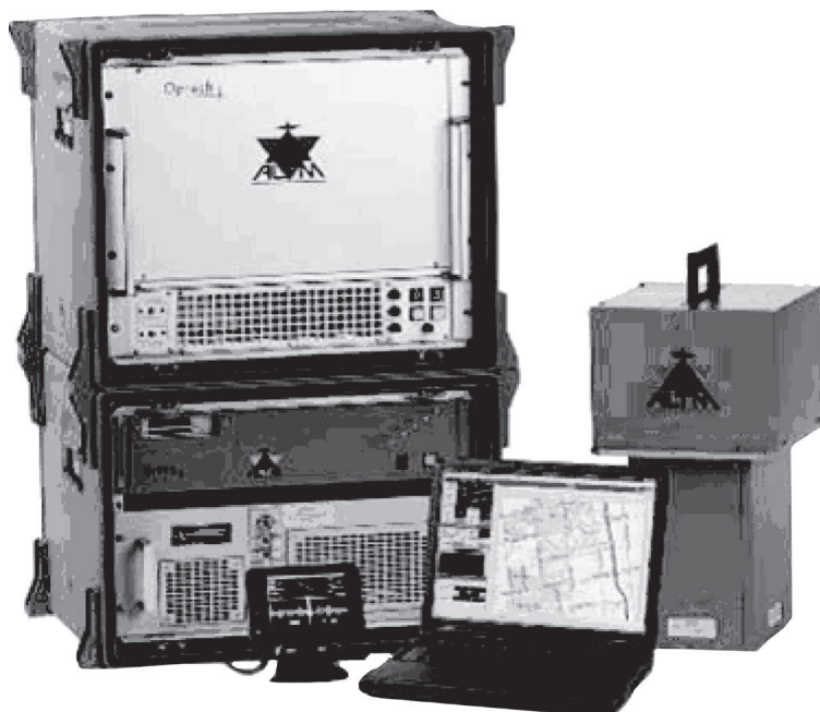
FIGURE 13.22 OPTECH 2050 LIDAR equipment operated by laser map
