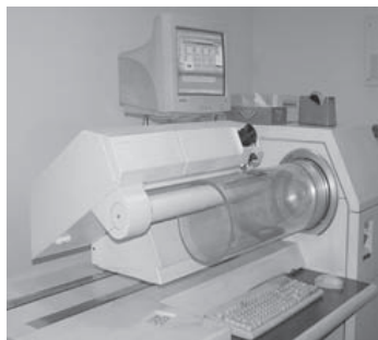
FIGURE 3.3 A drum scanner
