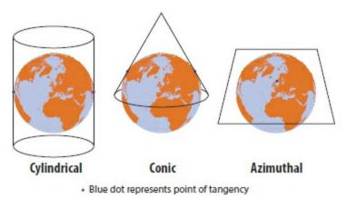
Common geometric shapes used to construct a map projection. Data from Data and Maps for ArcGIS 2010, courtesy of ArcWorld supplement and Esri.
