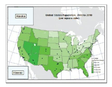
The map scale is changed to 1:20,000,000, and the layers are centered in the data frame. From here, you will begin the process of copying the data layers to the Hawaii and Alaska data frames.
