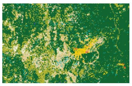
This raster of discrete data represents land cover. Data courtesy of Lake Tahoe Data Clearinghouse, US Geological Survey.
