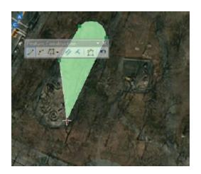
**11.** Switch to the End Point Arc Segment tool, and create another curved line to match the image layer. Click to finish the curved line.
