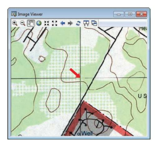
The second click links the ground control point to the real-world coordinate. Notice in the Link window that the first link has been created and that the X and Y Source values are the same (or very close to the same) as X and Y Map values. This happens because ArcMap does not yet know the real-world coordinates indicated on the map. You will change the X and Y Map values using information from the raster.
