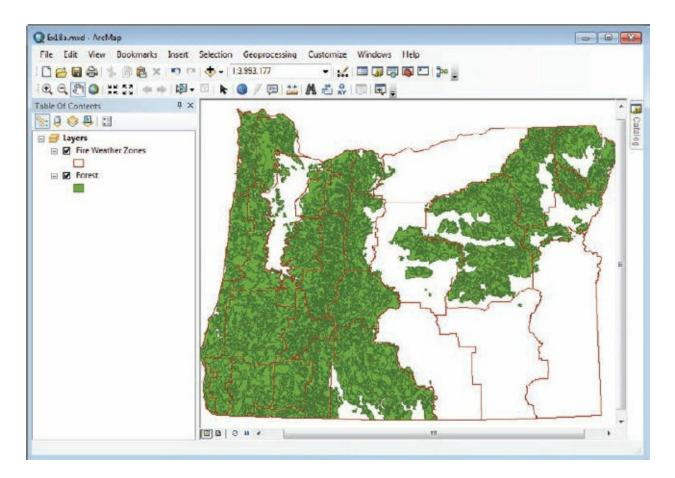
The map shows the Forest polygon layer and the Fire Weather Zones polygon layer symbolized by a dark-red outline and hollow fill—the hollow fill allows the zones to be overlaid on top of the forest layer without obscuring it.
