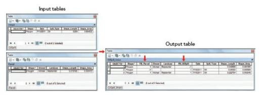
The output table contains the attributes of both input layers. Output features get the attribute values of input features with which they are spatially coincident.
