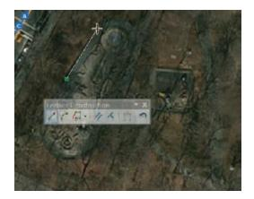
9. On the Feature Construction (or the Editor) toolbar, click the End Point Arc Segment tool *▼*. Click once to place a vertex on the eastern edge of the curved end. Then move your mouse northward to adjust the curvature of the line. Finally, click to create the curved line.
