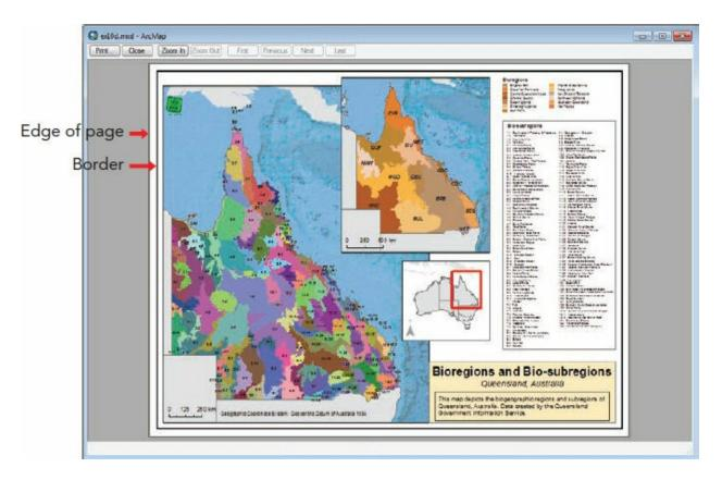
At this point, you should mainly be concerned with the alignment of the elements on the page. Your alignment will depend on the type of printer you are connected to and its configuration. If the map elements overlap the page edge, this problem can be corrected.
