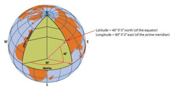
Angles are used instead of distance, because as meridians converge toward the poles, the distance between them decreases. A degree of longitude is about 69 miles near the equator, about 49 miles at the 45th parallel, and zero at the North Pole. In other words, distance varies between meridians, and only the angle between them remains constant. Data from Data and Maps for ArcGIS 2010, courtesy of ArcWorld supplement and Esri.
