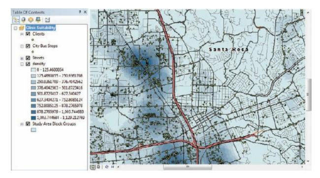
The Point Density tool created a raster surface that shows where points are clustered. The darker areas have a higher concentration of current clients, and the lighter areas have a lower concentration. Each client location was counted once.
