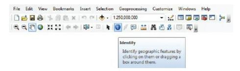
When you use the Identify tool, the pointer is accompanied by an *i* symbol as you move it around the map display. When you click a feature, it opens the Identify window.
