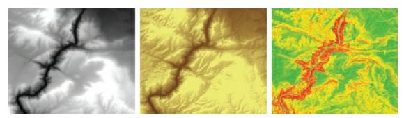
*Left to right*: Rasters of elevation, hillshade, and slope for the same area. Raster images based on the National Elevation Dataset courtesy of the US Geological Survey.
