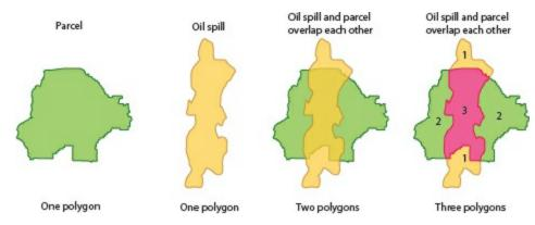
The parcel and oil spill layers are unioned to create three new polygons.
