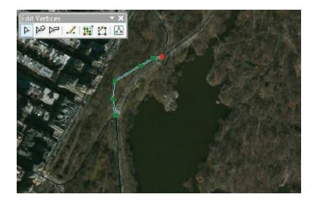
On the edit sketch, the vertices are green squares, and the end vertex is a red square. ArcMap has automatically activated the Edit Vertices toolbar. You can also activate the Edit Vertices toolbar by clicking the Edit Vertices button, which is now highlighted on the Editor toolbar.
