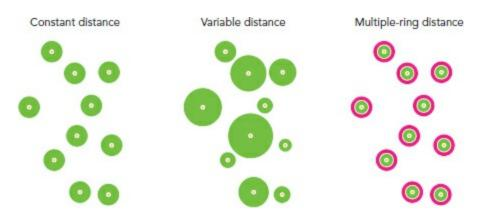
Buffers can be determined by distance in different ways.
