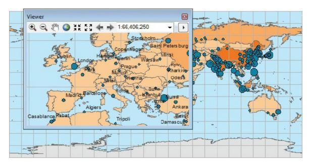
The Viewer window allows you to examine different parts of the map without changing the main display. You can move the Viewer window so it doesn't obscure the main map, or you can enlarge it—this is helpful when you have a large computer monitor (or two monitors) and you want to see two views of the same map simultaneously.
