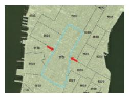
Because you are drawing the split line where adjacent polygon edges intersect the selected polygon, you shouldn't need to open the snapping toolbar because Intersection Snapping is turned on by default for every ArcMap session unless you turn it off.
