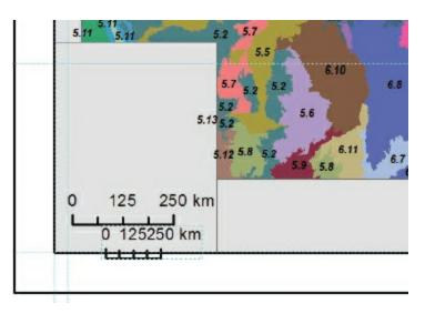
A second scale bar is added to the layout and placed near the Biosubregions scale bar. It doesn't look quite right because the Bioregions map scale (1:24,000,000) is different from the Bio-subregions map scale (1:13,000,000).
