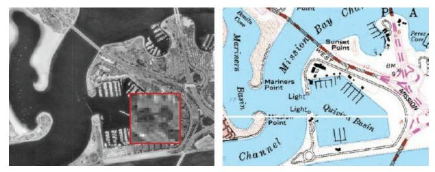
An air photo (*left*) and a scanned map (*right*) of the area around San Diego's Mission Bay. If you zoom in close enough on any raster, its cell structure will be revealed, as shown by the inset in the red box on the air photo. Satellite image and map courtesy of the US Geological Survey.
