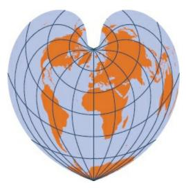
World Bonne is an equal-area projection that has true scale along the central meridian and all parallels. Shapes are distorted as you move away from these lines. Data from Data and Maps for ArcGIS 2010, courtesy of ArcWorld supplement and Esri.
