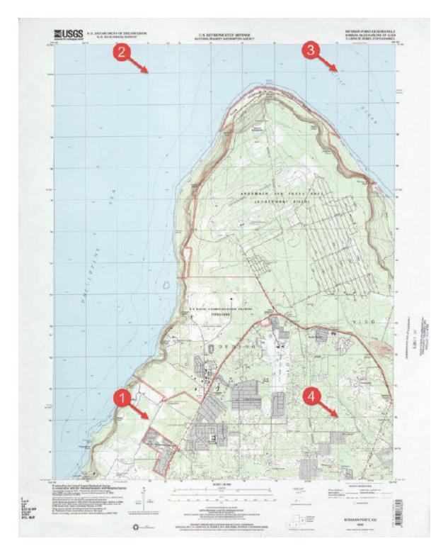
**13.** Using either the Image Viewer or the Data View of the main ArcMap window, click the intersection of the grid lines once to add the ground control point, and immediately click again in the same position. (If you moved the cursor to another position, right-click and click Cancel Point, and try again.)
