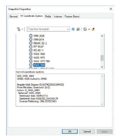
The Shapefile Properties dialog box shows that this layer has a geographic coordinate system called GCS\_WGS\_1984 (WGS 1984). It is another popular geographic coordinate system that is in wide use. Since it is different from the coordinate system of the US states layer, it may not align exactly. ArcMap, however, is designed to make it work.
