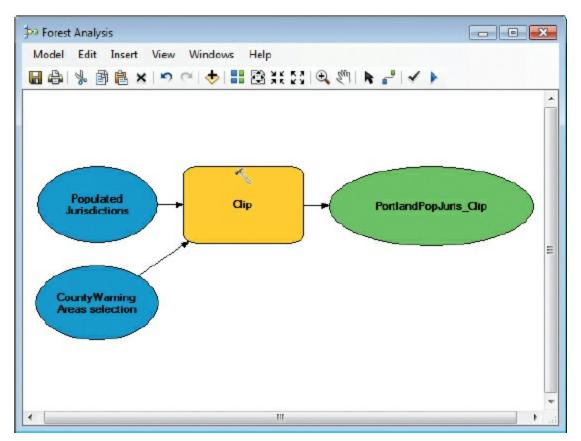
A model using the Clip tool in ModelBuilder.
