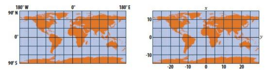
*Left*: A geographic grid with longitude values along the x-axis and latitude values along the y-axis. *Right*: On a flat map, coordinate values can represent any kind of linear unit. Data from Data and Maps for ArcGIS 2010, courtesy of ArcWorld supplement and Esri.
