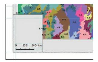
Next, you will insert an additional scale bar for the Bioregions data frame. This time, to speed up the process, you will copy the scale bar you just created and paste it when the Bioregions data frame is active. This is possible because the scale bar is dynamically linked to an active data frame. The values and width will adjust accordingly.
