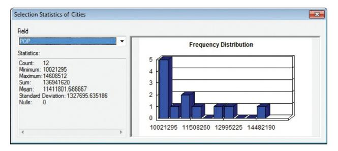
The statistics window displays the number of records for which statistics are being calculated (12) and the minimum, maximum, sum, mean, and standard deviation values.
