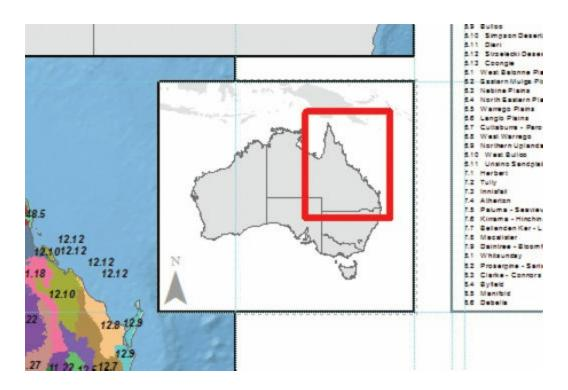
Next, you will add a scale bar to the Bio-subregions data frame. Scale bars tell you how to convert measurements on the map into the real distances they represent on the ground.
