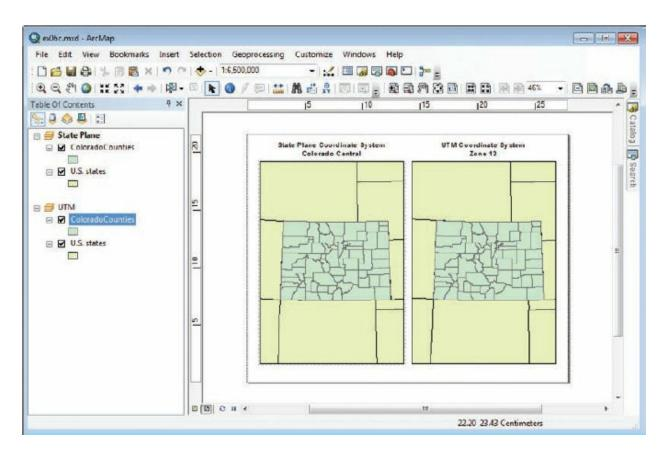
The Colorado counties layer is copied to the UTM data frame and is projected to UTM Zone 13. This is possible because the projected UTM coordinate system is also based on the GCS\_North\_American\_1983 geographic coordinate system.
