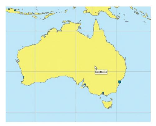
MapTips are a layer property. They can be turned on or off on the Display tab on the Layer Properties dialog box. You can see MapTips no matter which tool is active.
