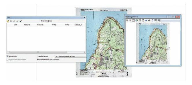
12. Using the graphic as a reference, use the Image Viewer and zoom into the intersection of the grid lines indicated by label 1. (The labels are just for reference and don't appear on the actual raster.) On the Georeferencing toolbar, click the Add Control Points button ∠.
