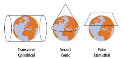
Variations of common geometric shapes create different map projections. Data from Data and Maps for ArcGIS 2010, courtesy of ArcWorld supplement and Esri.
