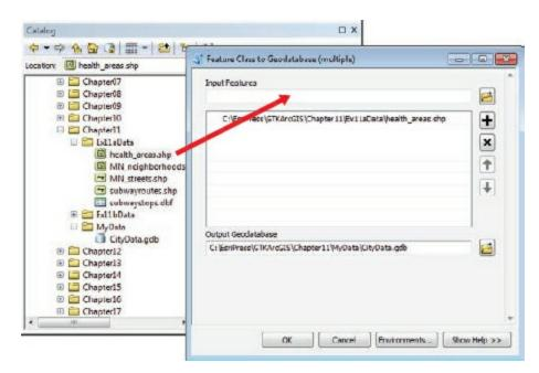
The path to the feature class is displayed in the Input Features box. In the Output Geodatabase box, Catalog correctly assumes you want to import the data into the CityData geodatabase. (You could change the output location if desired.)
