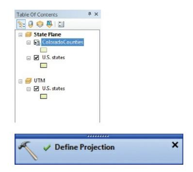
While the Define Projection tool is running, ArcMap locks the layer so it cannot be accidentally modified or moved. A notification indicates the process was successful. ArcMap projects the Colorado counties layer to the Colorado North State Plane Coordinate System projection. The State Plane data frame is updated, and the Colorado counties layer disappears from the map display.
