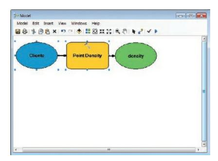
**10.** Run the model (on the model menu bar, click Model > Run). When the process is complete, right-click the density element in the model and click Add To Display. Be sure to keep your model open for the extent of this
