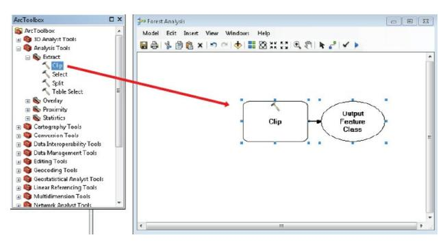
**14.** Click the Clip tool and drag it to the center of the model window.
