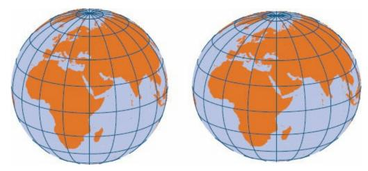
*Left*: Some geographic coordinate systems are based on the assumption that the earth is a sphere. *Right*: Most geographic coordinate systems are based on the assumption that the earth is a spheroid (exaggerated). The spheroid is a more accurate model because the earth bulges slightly at the equator and is flattened at the poles. Data from Data and Maps for ArcGIS 2010, courtesy of ArcWorld supplement and Esri.
