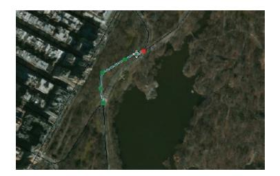
**11.** Use the pointer to drag the vertex down to the center of the road in the basemap, and then release the mouse button.
