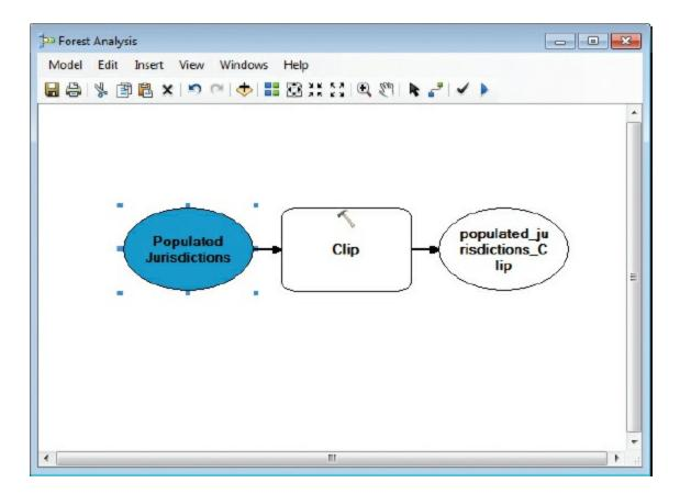
The Populated Jurisdictions layer, represented by a blue oval, is automatically connected to the tool it was dropped onto. Because clipping requires two layers, you will set the Portland CWA as a model parameter as well.
