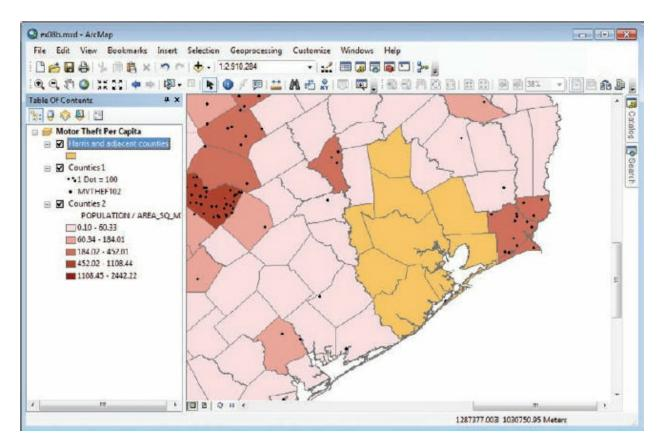
**14.** Open the Counties 1 properties. On the Symbology tab, click the Properties button. On the Dot Density Symbol Properties dialog box, select the Use Masking check box, select HarrisAdjacentCounties in the Control Layer list, and click the "Place dots only in these areas" option. Then click OK.
