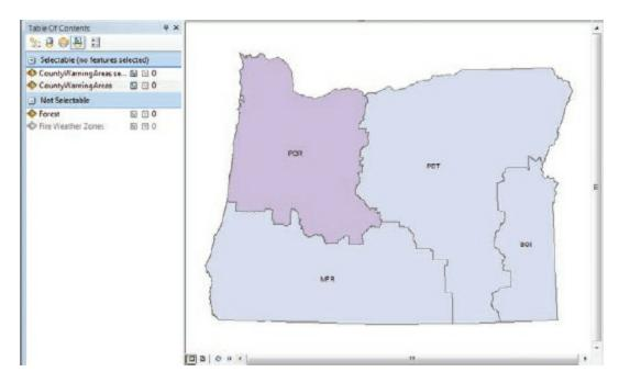
**7.** In the table of contents, click the List By Drawing Order button. Turn off the CountyWarningAreas layer and drag the CountyWarningAreas selection layer to the bottom of the table of contents.
