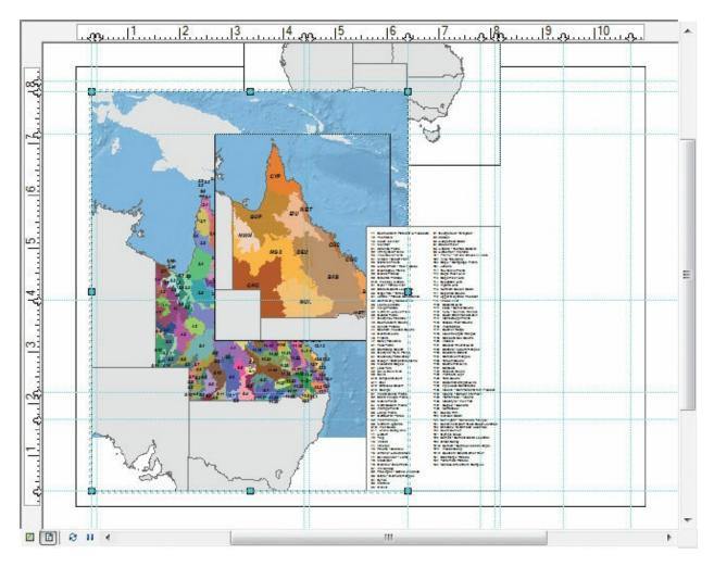
**14.** On the Standard toolbar, in the Map Scale box, replace the existing scale with **1:13,000,000**, and press Enter.
