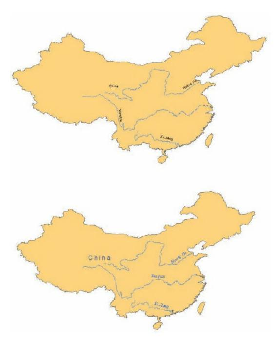
Default labels (*top*) are often sufficient, but you can modify the default labels (*bottom*) to improve the map's appearance by changing the font, color, size, character width, and spacing; adding special effects such as halos; or specifying placement settings, such as curving river labels along the lines of features. You can also choose from many predefined label styles offered in ArcMap. Data from Data and Maps for ArcGIS 2010, courtesy of ArcWorld and ArcWorld Supplement.
