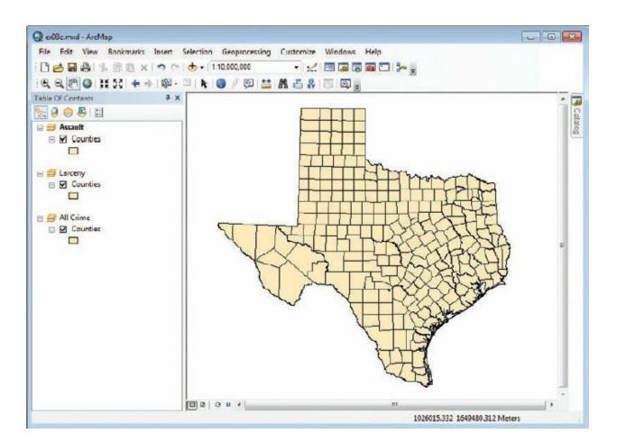
The map is open in data view. In the table of contents, there are three data frames: Assault, Larceny, and All Crime. Each data frame has a Counties layer (all from the same data source). The Assault data frame is active.
