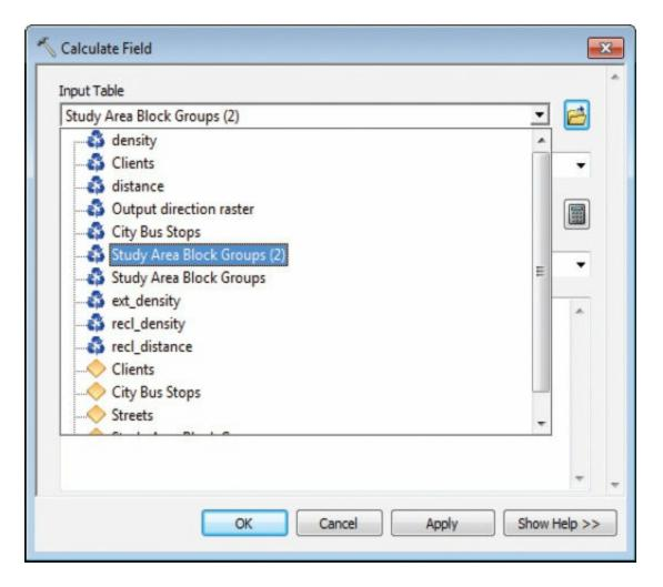
Intermediate data means the layers that reside in the model, rather than those that reside in the map document. In other words, the new field can't be calculated until it has been added, so the Calculate tool now knows to do its work on the new Study Area Block Groups layer that is created as an output of the Add Field operation.
