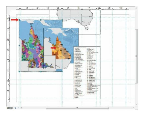
Next, you will make the Bio-subregion's data frame bigger by dragging a selection handle. When you resize a data frame, ArcMap automatically adjusts the **map extent** and the display scale.
