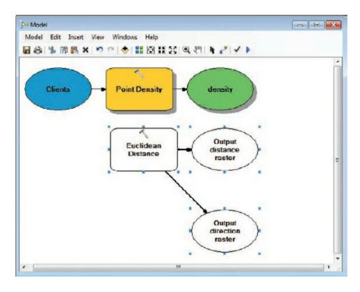
You want to calculate the distance from bus stops. You aren't interested in areas that are farther than a half-mile walk from a bus stop (and the most desirable areas will be much closer than that), so you will choose a maximum output distance of a half mile (2,640 feet).
