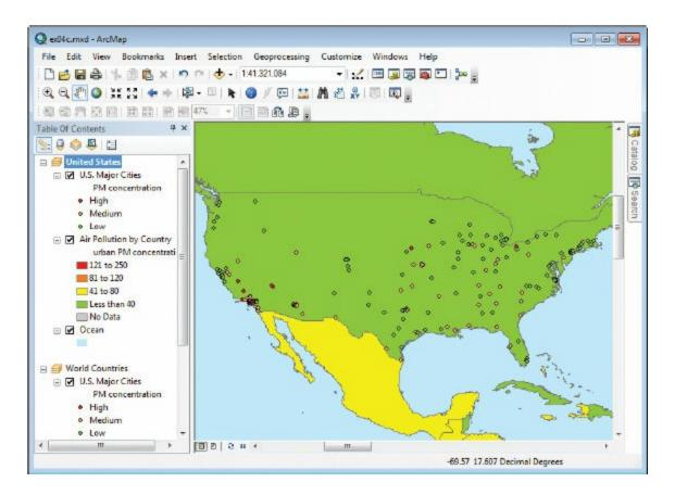
The display window shows the contents of the active data frame. The name of the active data frame is in boldface in the table of contents. In the graphic, the active data frame is called United States. The default name given to data frames is Layers.
