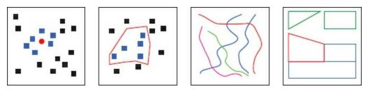
*Left to right*: Points within a given distance of the red point are selected, points contained by the red polygon are selected, lines that intersect the red line are selected, and polygons adjacent to the red polygon are selected.
