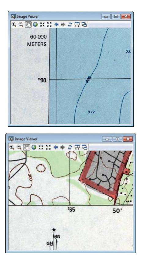
The bottom boundary grid line value is listed as 265—in UTM units, this means it is 265,000 meters. The left boundary grid line value is listed as 1500
