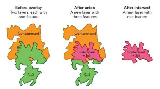
*Left*: An area of soil and a spilled contaminant zone overlap each other. Overlay analysis—whether union (*center*) or intersect (*right*)—creates new features where input layers overlap
