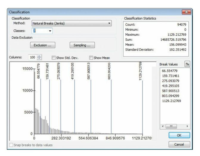
The output will have seven (7) classes, with the highest number (7) assigned to the areas that have the highest density of existing clients.
