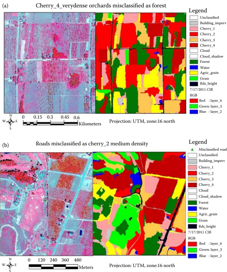
FIGURE 17.3 (a) left is color infrared, and right is an eCognition segmented classification. Toward the center of the image is an area of very dense cherry orchards that were misclassified as forest. (b) left is color infrared, and right is an eCognition segmented classification. Toward the center of the image is an area of roads, lined with trees, that were misclassified as Cherry_2 medium density.
