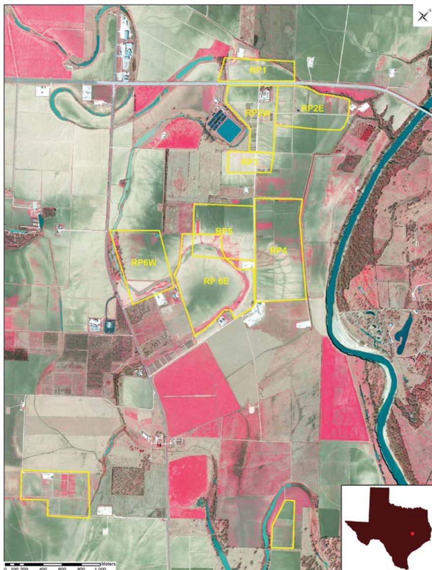
FIGURE 1.1 False-color composite (green, red, NIR) orthoimagery over the study area in Burt County, Texas. The Brazos River is on the right of the image, and the FM 60 highway runs left to right near the top of the image and crosses the Brazos River. Data collection was attempted in one UAS flight in route packs (RPs), outlined in yellow. The 6-in and 12-in 4-band (blue, green, red, NIR) orthoimageries were acquired between January and February 2013 during leaf-off conditions. The data set covers approximately 1963 km 2 (758 mi 2 ). Five local entities contributed funds to collect the new imagery using the High Priority Imagery and Data Sets (HPIDS) State contract administered by the Texas Natural Resource Information System (TNRIS) Strategic Mapping Program (StratMap).
