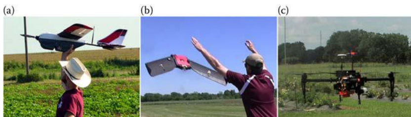
FIGURE 1.2 Select UASs evaluated in this study: (a) PrecisionHawk Lancaster 5 with Nikon 1 J4 visual camera; (b) Tuffwing UAV Mapper with Sony A6000 visual camera; and (c) DJI Matrice 100 with MicaSense RedEdge multispectral camera.
