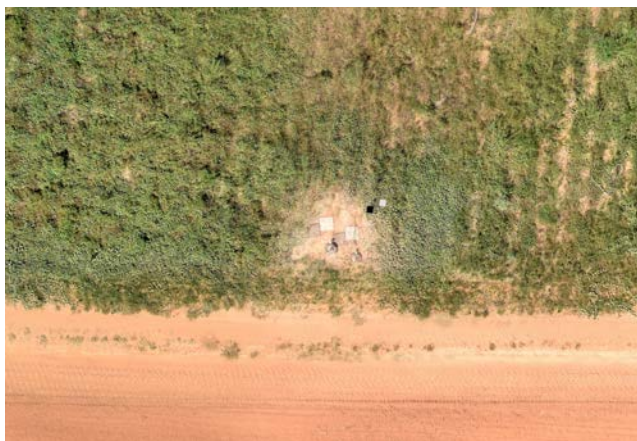
FIGURE 1.4 Orthoimage with overall subpixel RMS error, but with duplication and mislocation errors of \sim 25 pixels due to inclusion of images with excessive aircraft roll. Note ghostly white and dark gray concrete tiles (GCPs). True locations given by black and white squares.
