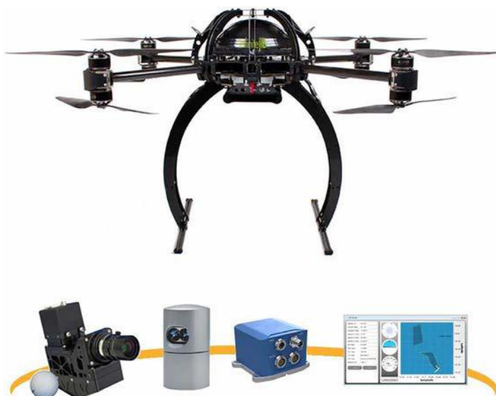
FIGURE 3.8 Typical components of a hyperspectral UAV.
