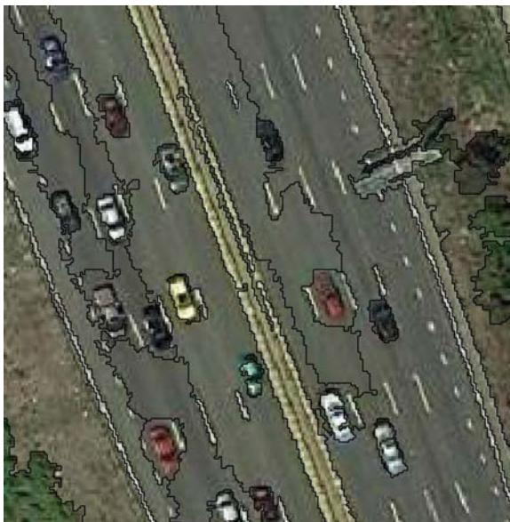
FIGURE 10.4 Segmentation results of a road with several cars where object boundaries are delineated by black lines.
