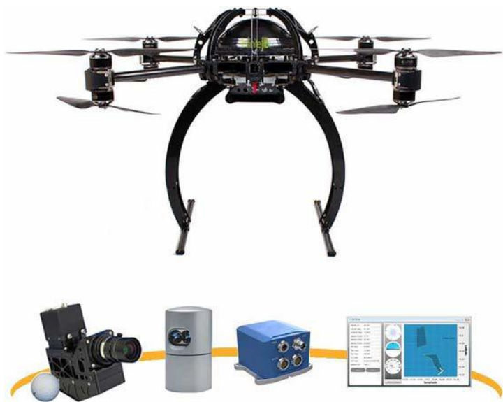
FIGURE 3.8 Typical components of a hyperspectral UAV.
