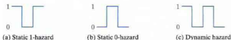
FIGURE 9.34 Types of hazards
