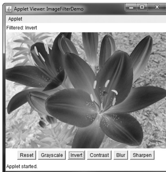
Figure 27-7 Using the Invert filter with ImageFilterDemo
