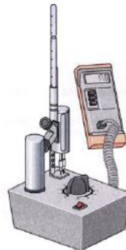
An instrument used to measure melting point.
