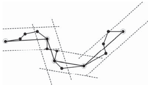
Figure 7.20: Example of reducing lines by the use of corridor. The numbers of points needed to describe a line are reduced by moving forward a corridor of a given width until it touches the digitized line. All the points on the line in the corridor, apart from the first and last, are deleted. This process is repeated until the entire line is trimmed.
