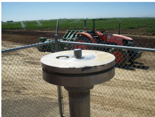
Fig. 6.4 Antenna mount without a GNSS antenna
