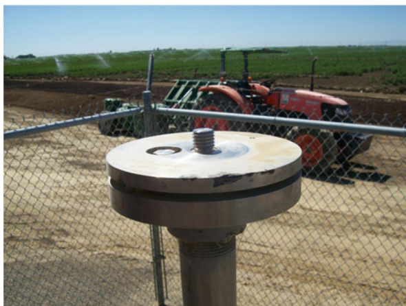
Fig. 6.4 Antenna mount without a GNSS antenna
