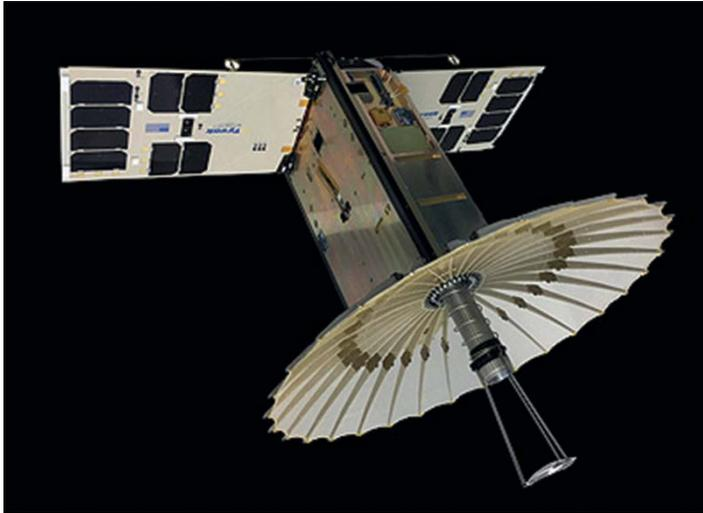
Figure 9.23 Picture of the Rain Cube satellite.
