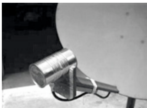
Figure 4.10: Feed horn made from a food can.
