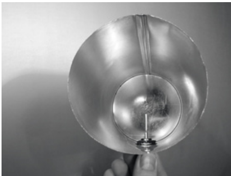
Figure 4.41: Your finished cantenna.
