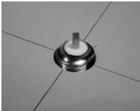
Figure 4.22: The N connector should fit snugly in the hole.
