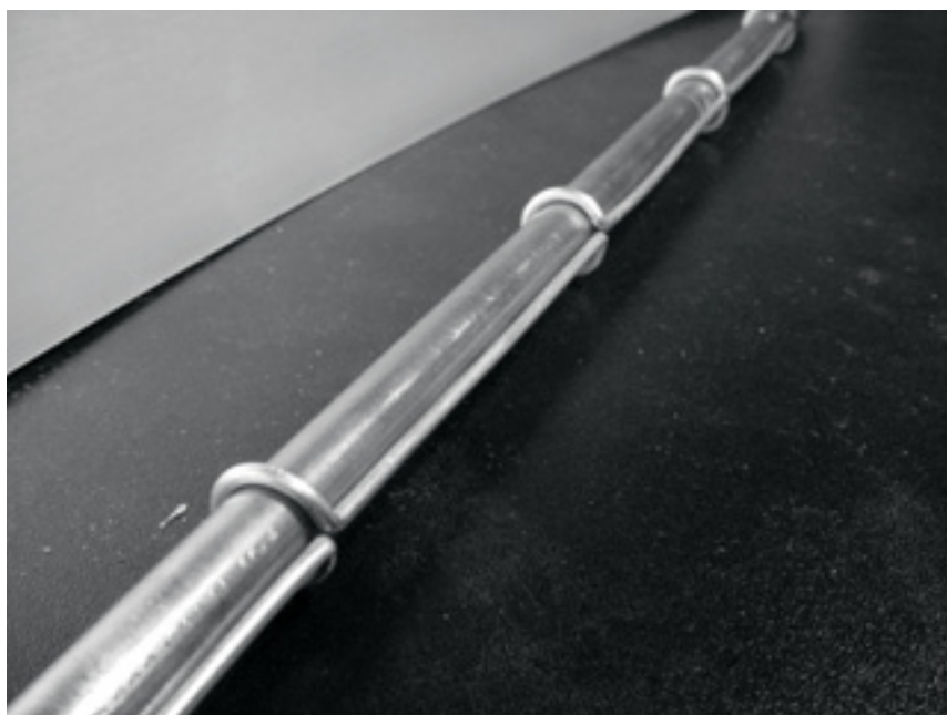
Figure 4.20: Inserting a pipe can help to straighten the wire.
