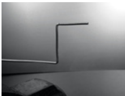
Figure 4.16: Bend the wire into a "Z" shape.
