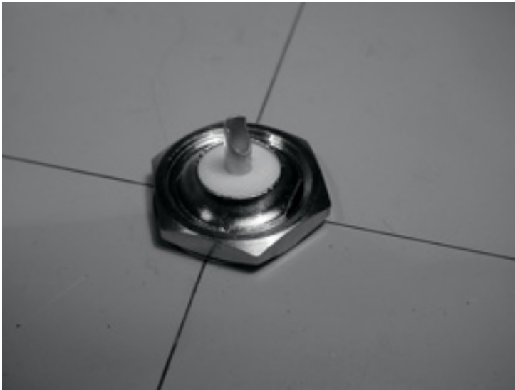
Figure 4.24: Secure the N connector tightly to the plate.
