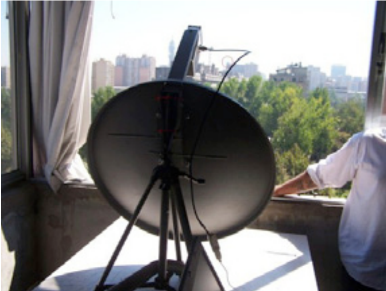
Figure 11.17: Wireless station and parabolic antenna used for the transmission of Santiago-2006 FLISOL via streaming video.
