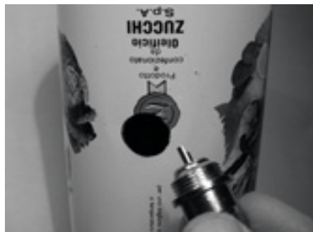
Figure 4.36: Carefully drill a pilot hole, then use a larger bit to finish the job.
