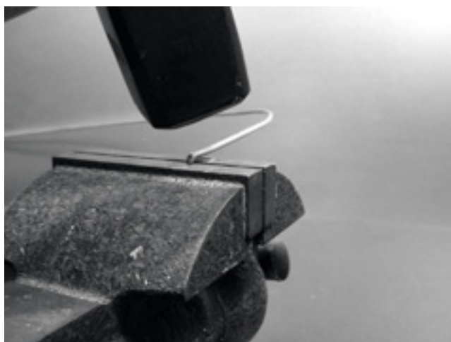
Figure 4.15: Gently tap the wire to make a sharp bend.
