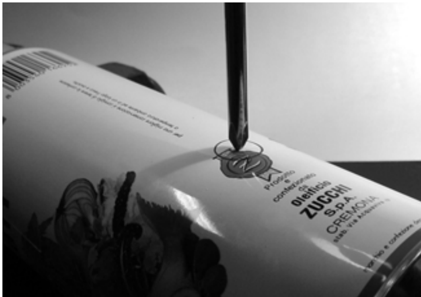
Figure 4.35: Mark the hole before drilling.
