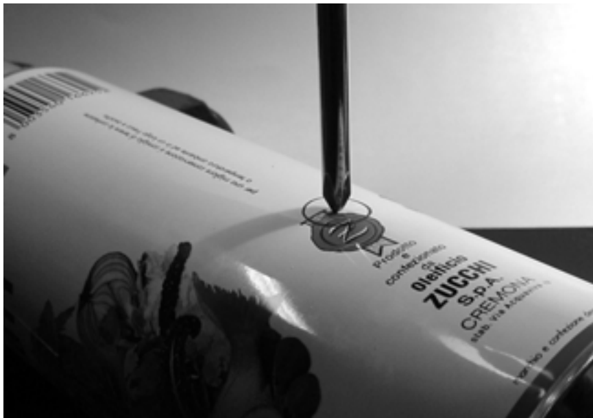
Figure 4.35: Mark the hole before drilling.
