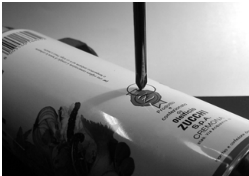
Figure 4.35: Mark the hole before drilling.
