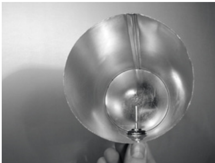
Figure 4.41: Your finished cantenna.
