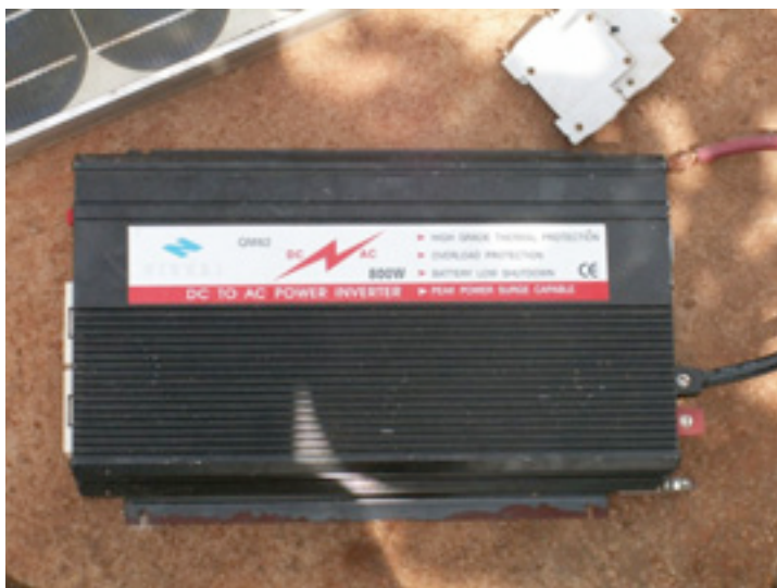
Figure 7.4: An 800 Watt DC/AC converter (power inverter)
