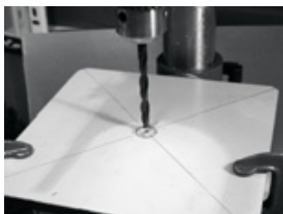
Figure 4.21: Drilling the hole in the metal plate.
