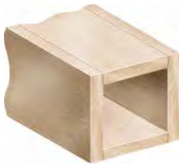
Wooden box beam
