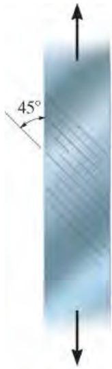
Lüder's lines on mild steel strip
