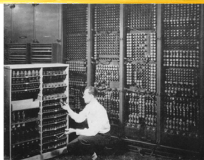
Replacing a bad tube meant checking among ENIAC's 19,000 possibilities.
