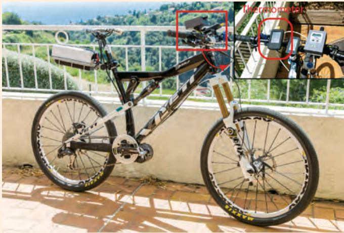
Figure 2 Bike with sensors for mobile temperature measurements. Photo: Martin, 2015.
