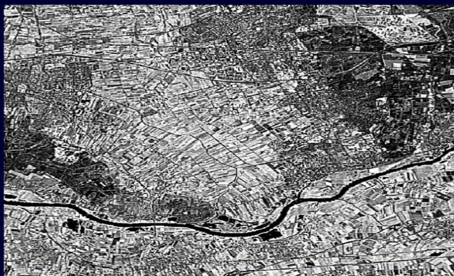
Result high pass filter, 3x3 window
