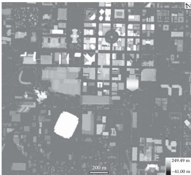
FIGURE 3.9 DHM raster created from DSM and DTM.
