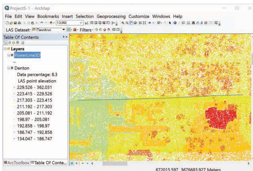
FIGURE 5.25 LiDAR dataset and a simulated powerline in Denton, TX, USA.
