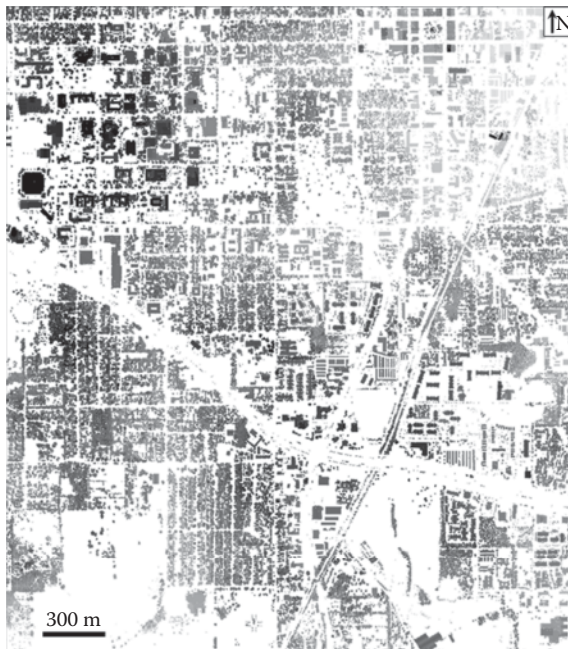
FIGURE 5.3 Non-ground DSM derived from LiDAR data.
