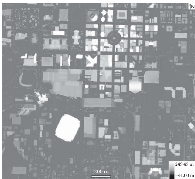
FIGURE 3.9 DHM raster created from DSM and DTM.
