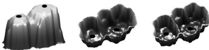
FIGURE 4.15 Marker-controlled watershed segmentation. (Left) CHM, (middle) inverted CHM, (right) inverted CHM with dam built to separate the watersheds. Dark markers are treetops. (Adapted from Chen, Q. et al., Photogramm. Eng. Remote Sens. , 72, 923–932, 2006.)
