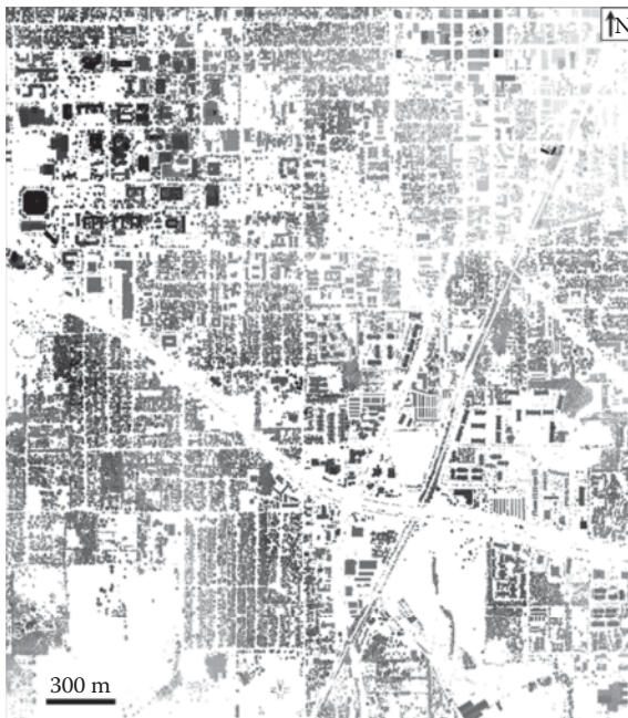
FIGURE 5.3 Non-ground DSM derived from LiDAR data.
