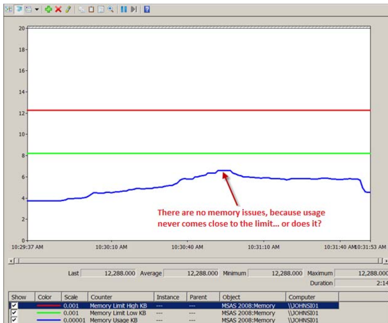
Figure 45 - Memory measurements with scaled counters
