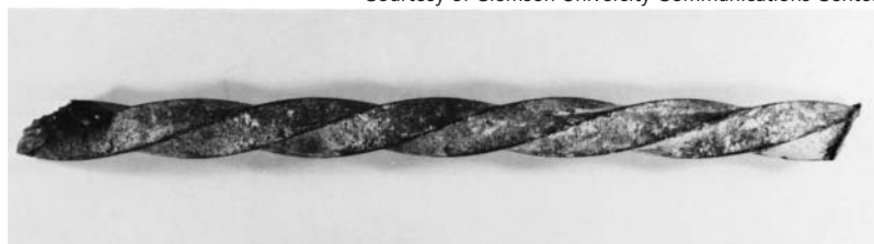
Twisted square bar, formerly used to increase bond between concrete and steel.
