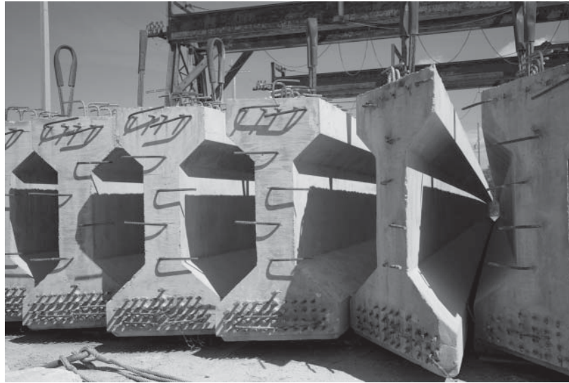
Precast prestressed highway bridge girders at production facility in central Florida.
