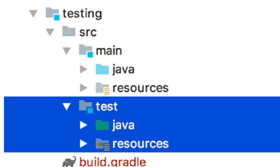
Figure 9-13. The Gradle module structure
