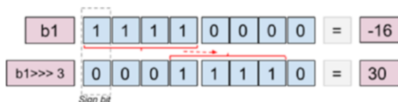
Figure 6-8. The effect of the >>> operator
