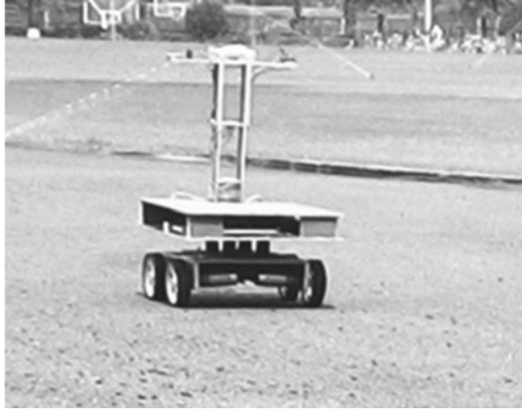
Fig. 4 The UMMS to acquire the geospatial data from inaccessible areas
