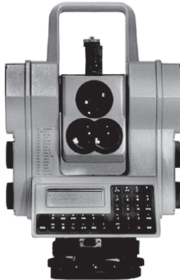
FIGURE 8.3 An old model total station
