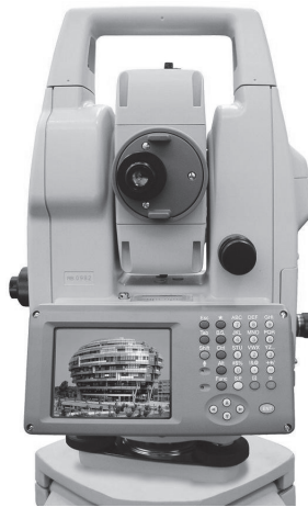
FIGURE 8.12 An imaging total station (courtesy of Sokkia)
