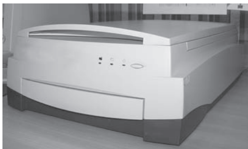
FIGURE 3.4 A flatbed scanner
