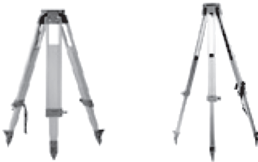
FIGURE 8.5 Wooden and aluminium tripods for total station
