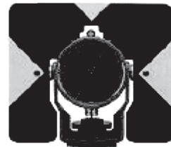
FIGURE 8.6 Typical standard prism and sight
