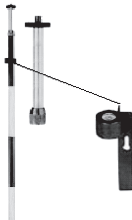
FIGURE 8.7 Typical standard rod (with bubble level)
