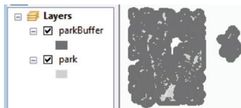
Figure 1.4 Input ( light gray ) and buffer output ( dark gray ) from script Example 1.1 with the input added to the map manually.
