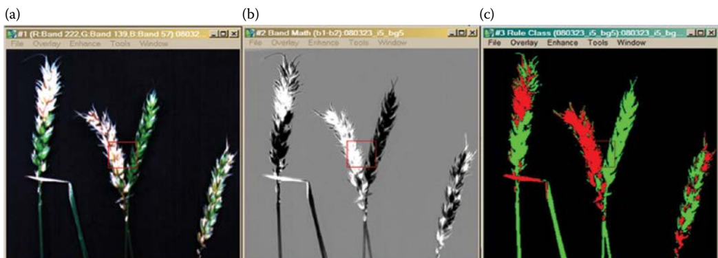
FIGURE 1.8 Examples of image classification of Fusarium -infected wheat ears. (a) RGB image, (b) grayscale image according to head blight index, (c) classification result (dark gray/red: diseased, light gray/green: healthy). (From Bauriegel, E. et al. 2011a. Computers and Electronics in Agriculture , 75, 304–312.)
