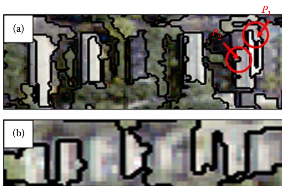
FIGURE 10.5 Comparison of two sets of buildings with (a) strong and (b) weak surrounding contrasts, and their segmentation results at the same scale.
