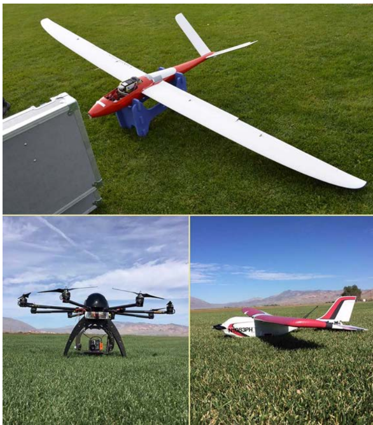
FIGURE 3.9 Examples of fixed-wing and octocopter hyperspectral UAVs.
