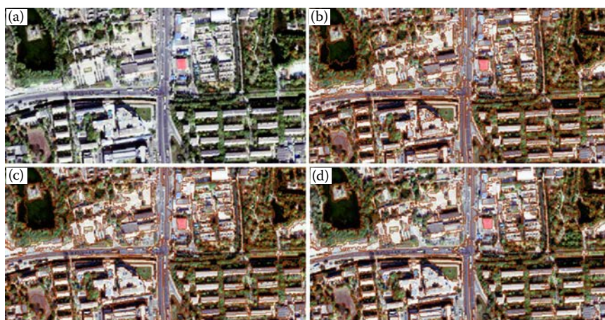
FIGURE 10.8 (a) Subimage of the study area, and three segmentation results based on different scale parameters of (b) 39, (c) 50, and (d) 66.
