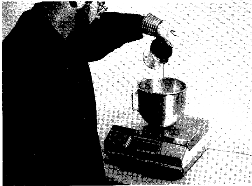
Figure 2.8 – Adding asphalt to heated aggregate
