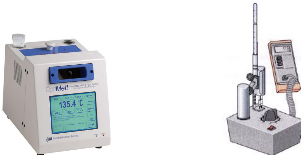
An instrument used to measure melting point.
