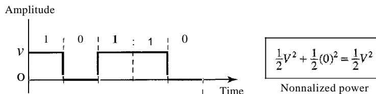
Figure 4.5 Unipolar NRZ scheme
