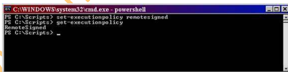
Figure 4: Setting the Execution Policy is as easy as running the set-execution policy command.
