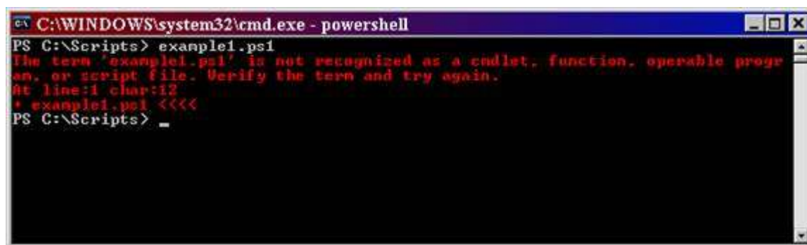
Figure 1: Scripts must include the path to the script to run successfully
