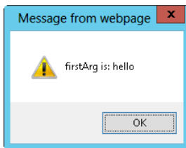
FIGURE 7-1 Using the arguments object within a function to access the first argument.
