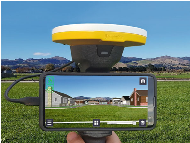
Fig. 1.2 A geodetic GNSS-based augmented reality system comprised of a geodetic antenna+receiver, data communication cable, and a mobile device with a display, camera, inertial orientation sensors, and other components. Image used by permission. Courtesy of Trimble Inc
