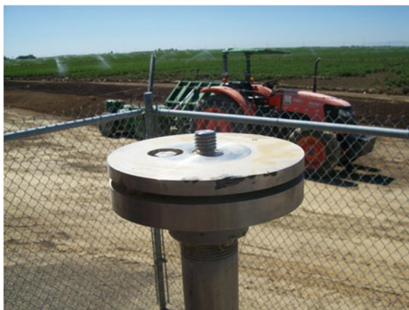
Fig. 6.4 Antenna mount without a GNSS antenna
