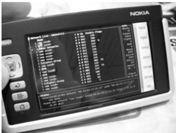
Figure 6.12: Kismet running on a Nokia 770 Internet Tablet
