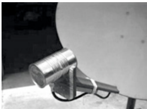
Figure 4.10: Feed horn made from a food can.
