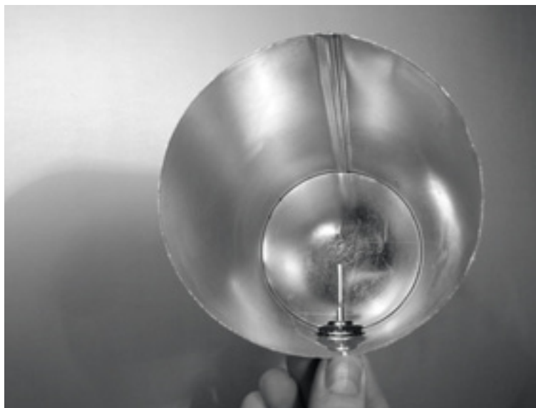
Figure 4.41: Your finished cantenna.
