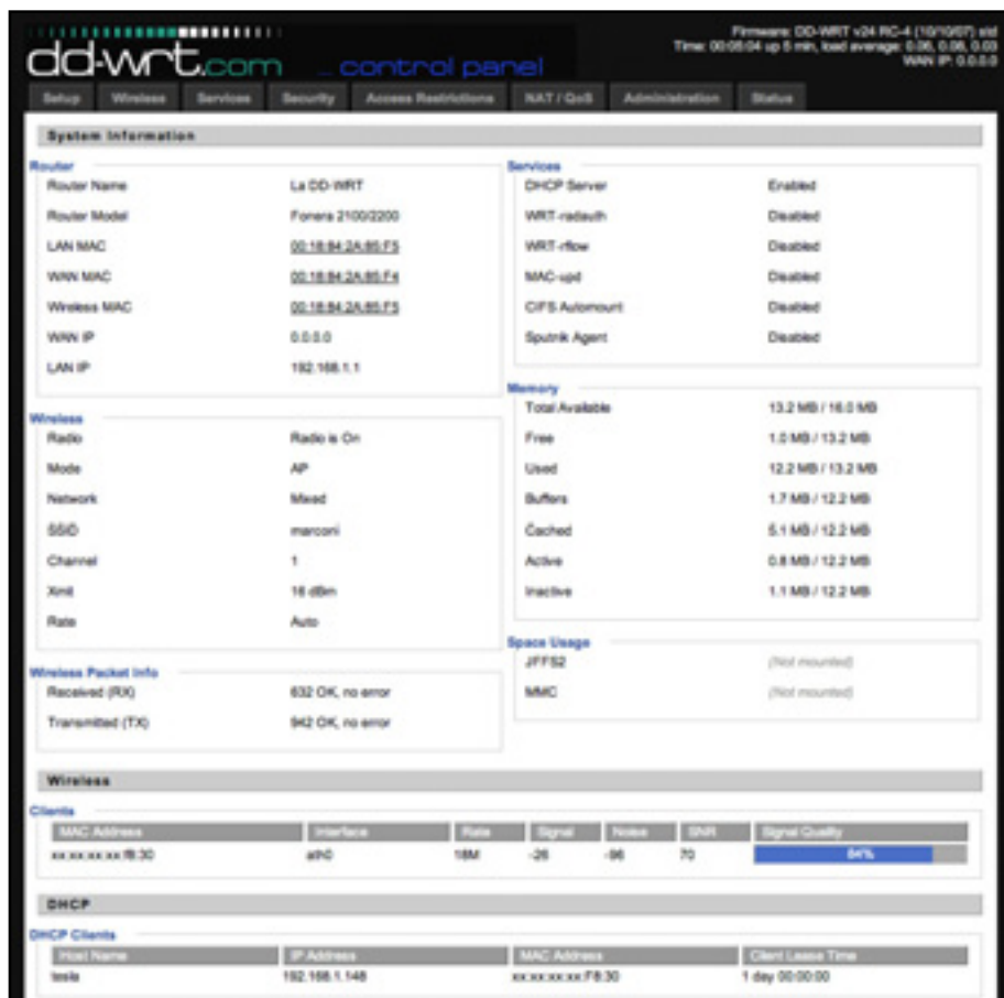
Figure 5.3: The DD-WRT (v23) control panel
