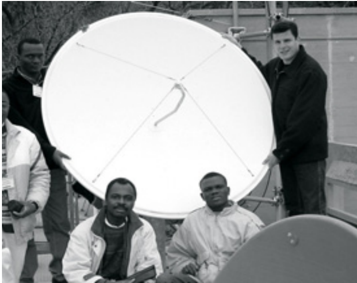
Figure 4.11: A solid dish antenna.
