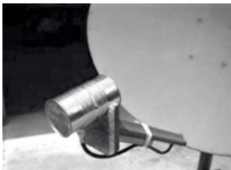
Figure 4.10: Feed horn made from a food can.
