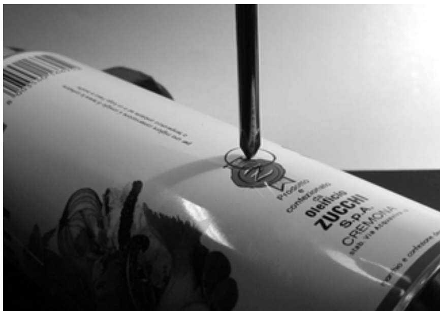
Figure 4.35: Mark the hole before drilling.
