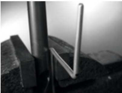
Figure 4.17: Bend the wire around the drill bit to make a coil.
