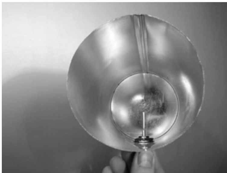
Figure 4.41: Your finished cantenna.
