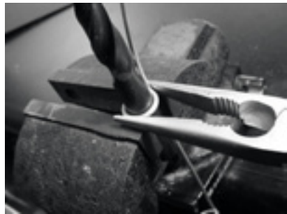
Figure 4.17: Bend the wire around the drill bit to make a coil.
