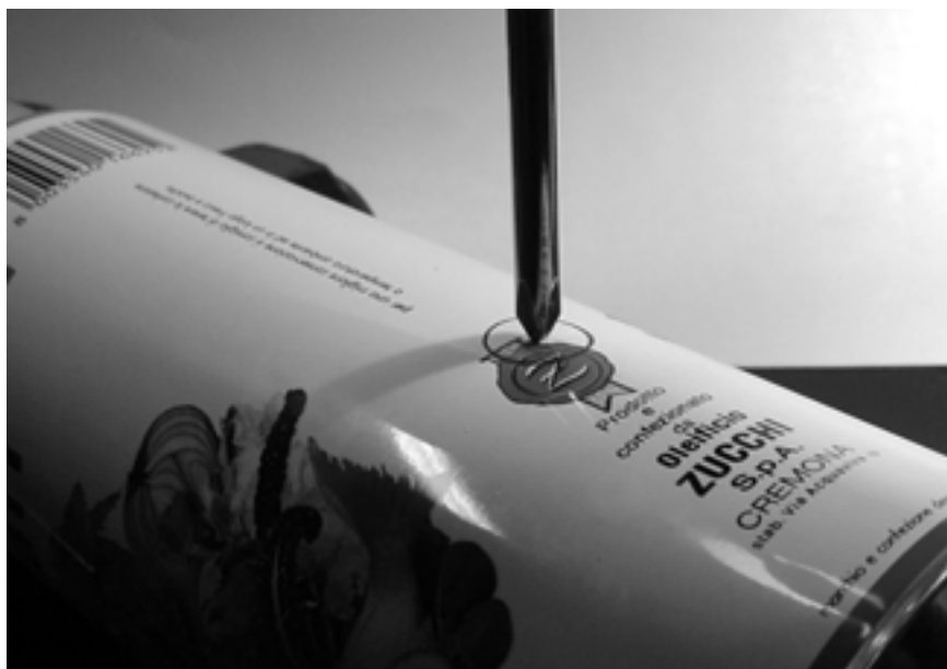
Figure 4.35: Mark the hole before drilling.
