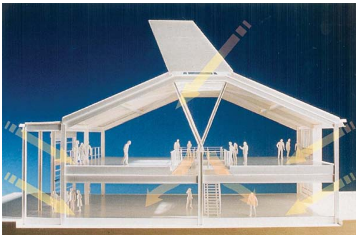
Section of model to illustrate the daylighting
