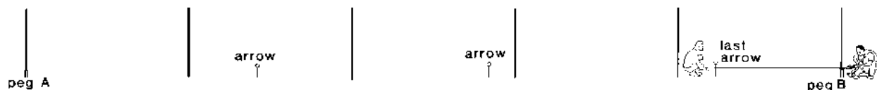
Fig. 16c Measurement of a long distance, Step 4
