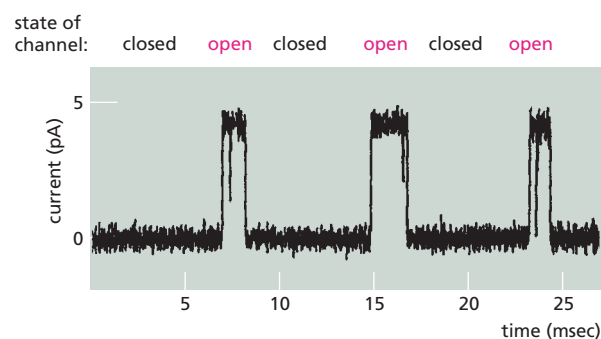
Figure 12–25 The behavior of a single ion channel can be observed using the patch-clamp technique. The voltage (the membrane potential) across the isolated patch of membrane is held constant during the recording. In this example, the neurotransmitter acetylcholine is present, and the membrane patch from a muscle cell contains a single channel protein that is responsive to acetylcholine (discussed later, see Figure 12–41). As seen, this ion channel opens to allow passage of positive ions when acetylcholine binds to the exterior face of the channel. But even when acetylcholine is bound to the channel, as is the case during the three channel openings shown here, the channel does not remain open all the time. Instead, it flickers between open and closed states. Note that how long the channel remains open is variable. If acetylcholine were not present, the channel would only rarely open. (Courtesy of David Colquhoun.)
