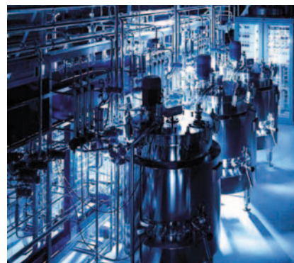
Figure 4–50 Biotechnology companies produce mass quantities of useful proteins. Shown in this photograph are the fermenters used to grow the cells needed for such large-scale protein production. (Courtesy of Bioengineering AG, Switzerland.)
