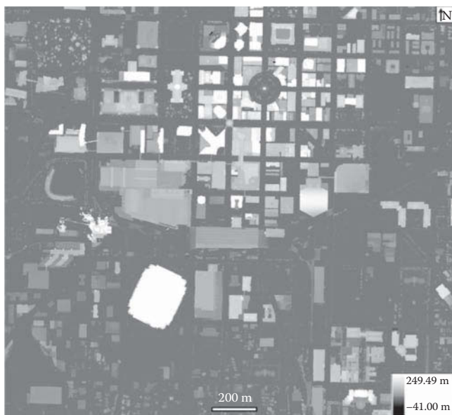
FIGURE 3.9 DHM raster created from DSM and DTM.
