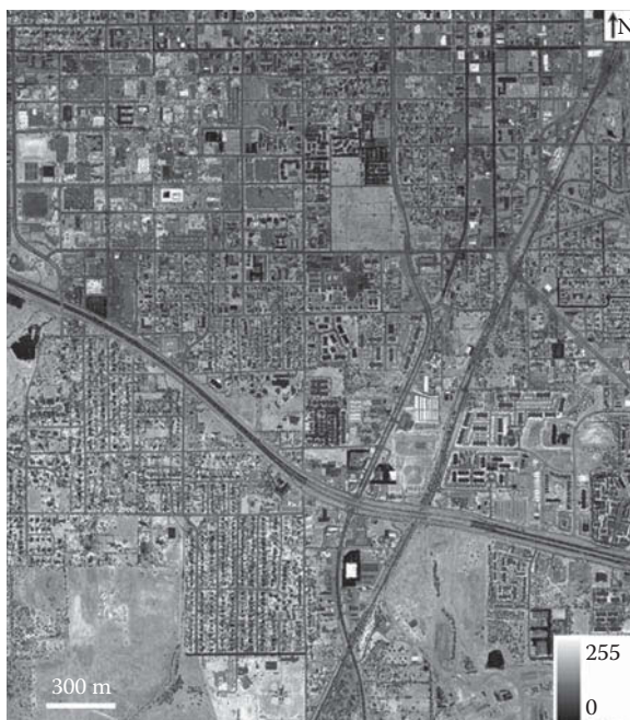
FIGURE 5.2 LiDAR intensity image for an area in Denton, TX, USA.
