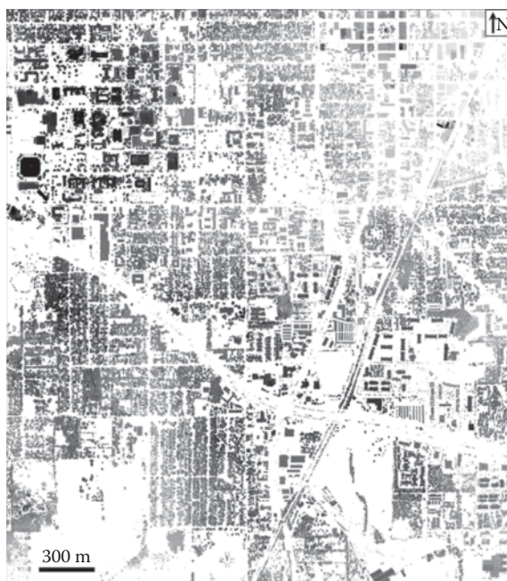
FIGURE 5.3 Non-ground DSM derived from LiDAR data.
