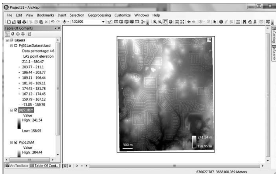
FIGURE 5.29 DSM created using LAS dataset to raster conversion.
