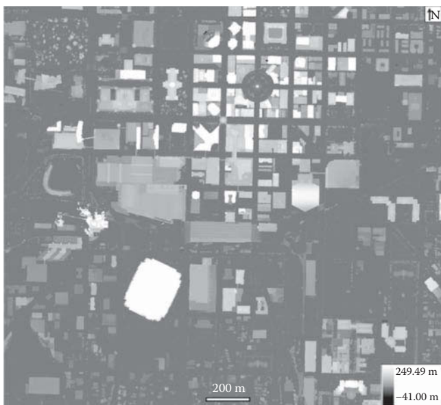
FIGURE 3.9 DHM raster created from DSM and DTM.
