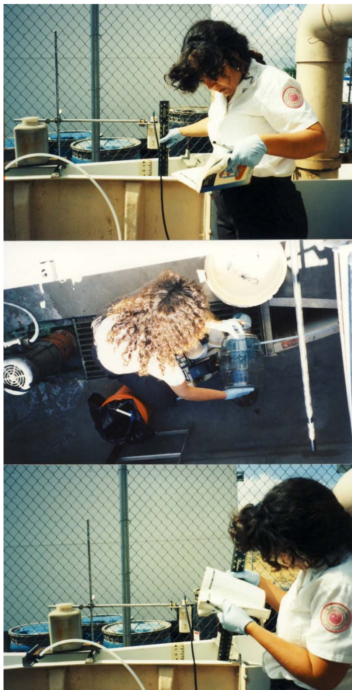
Here is a wastewater Inspector is utilizing the auto sampler's manual to help adjust the time and adjust for the correct flow for a composite sample. You can see that she is pouring off the pickle jar.
