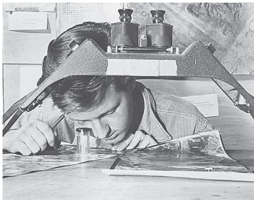
**FIGURE 5.13.** Image interpretation equipment, Korean conflict, March 1952. A U.S. Air Force image interpreter uses a tube magnifier to examine an aerial photograph in detail. A mirror stereoscope is visible in the foreground. From U.S. Air Force, U.S. National Archives and Records Administration, ARC 542277.
