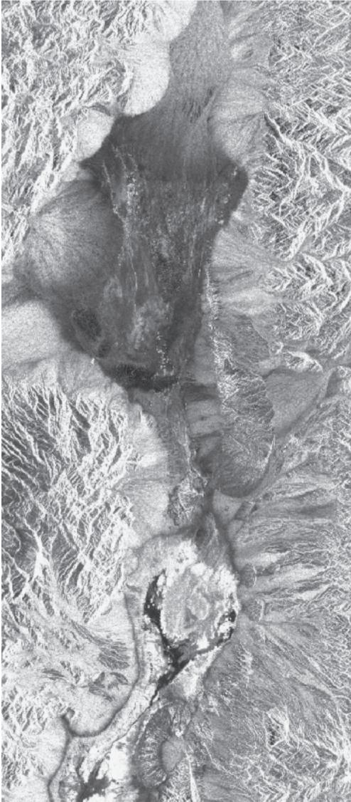
**FIGURE 7.7.** Image illustrating radar foreshortening, Death Valley, California. The unnatural appearance of the steep terrain illustrates the effect of radar foreshortening, when a radar system observes high, steep topography at steep depression angles. The radar observes this terrain from the right—radar foreshortening creates the compressed appearance of the mountainous terrain in this scene. From NASA-JPL; SIR-C/X-SAR October 1994. P43883.
