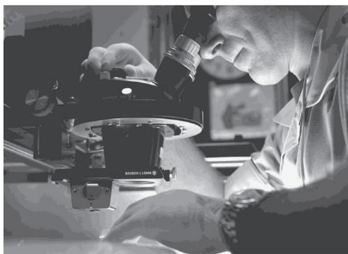
**FIGURE 5.14.** Binocular stereoscopes permit stereoscopic viewing of images at high magnification. From U.S. Air Force.
