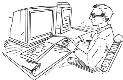
**FIGURE 5.18.** Digital photogrammetric workstation. The operator is depicted using polarizing stereovision glasses.
