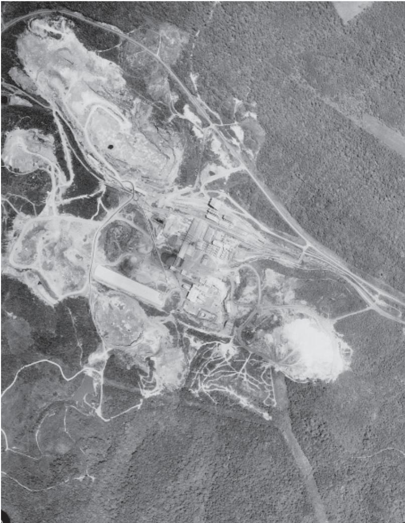
**FIGURE 20.12.** Delineation of the entire area devoted to a given use. This quarry consists of a complex of individual activities that together constitute a single enterprise, so the individual components need not be delineated separately. Copyright Virginia Department of Transportation. Used by permission.
