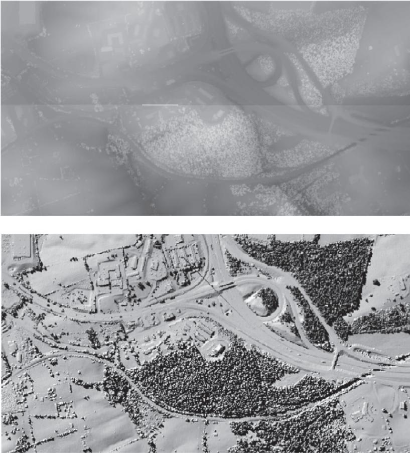
**FIGURE 8.6.** Section of a lidar image enlarged to depict detail. Upper image: raw lidar data, with brightness indicating increasing relative elevation. Lower image: lidar data processed with a hill-shading algorithm, revealing terrain texture; Wytheville, VA. From Virginia Department of Transportation. Copyright 2003, Commonwealth of Virginia. Reproduced by permission.
