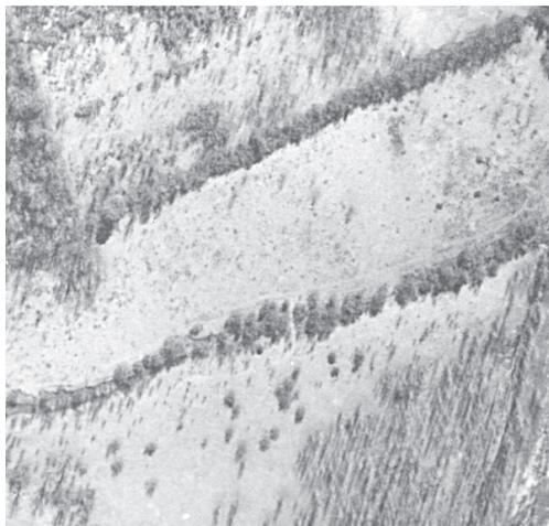
**FIGURE 5.5.** Significance of shadow for image interpretation, as illustrated by the characteristic pattern caused by shadows of shrubs cast on open field. Shadows at the edge of a forest enhance the boundary between two different land covers. From USDA.
