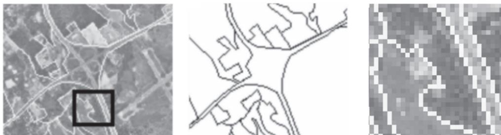
**FIGURE 5.17.** A digital record of image interpretation, showing the outlines as traced by the analyst using onscreen digitization (left), the outlines without the image backdrop (center), and a detail of the raster structure of the digitized outlines (right).
